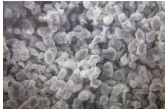
Picture 3: SEM, 1000X (only TiB<sub>2</sub>-crystals)
