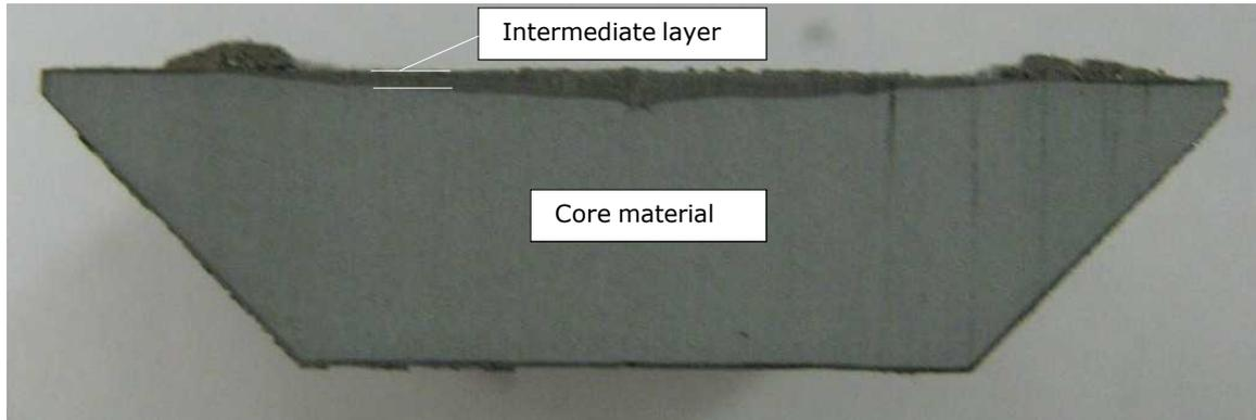
Picture 4: Cross section; used IMC evaporator
