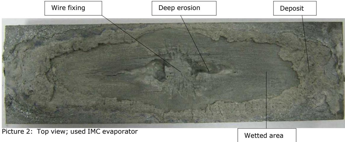
Picture 2: Top view; used IMC evaporator
