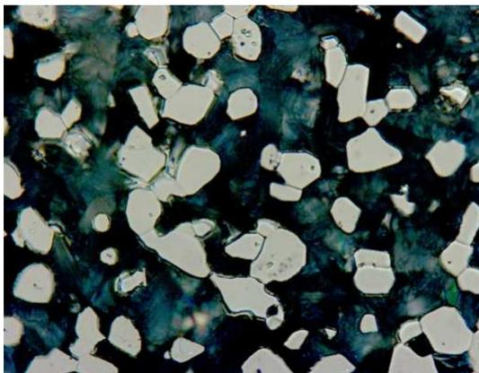
Picture 1: Heterogeneous mixture of BN and TiB<sub>2</sub> after hot pressing process
