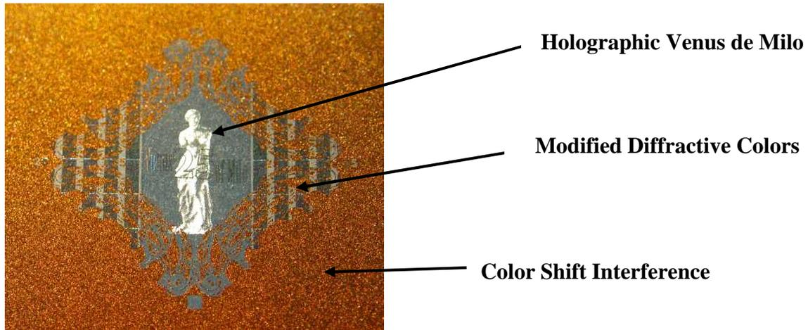
Fig. 3. Hybrid Device of Holographic and Thin Film Interference Elements
