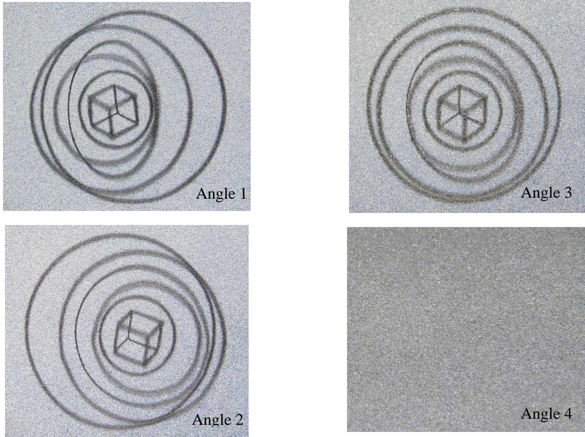
Fig. 4. 3D Floating Virtual Images above an Array of Glass Beads
