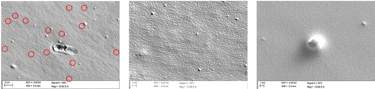
*Figure 2 – SEM images of plain film surfaces (10 000x magnification) – left to right: BOPP A ('dimples' marked by circles), BOPP B, BOPP C*
