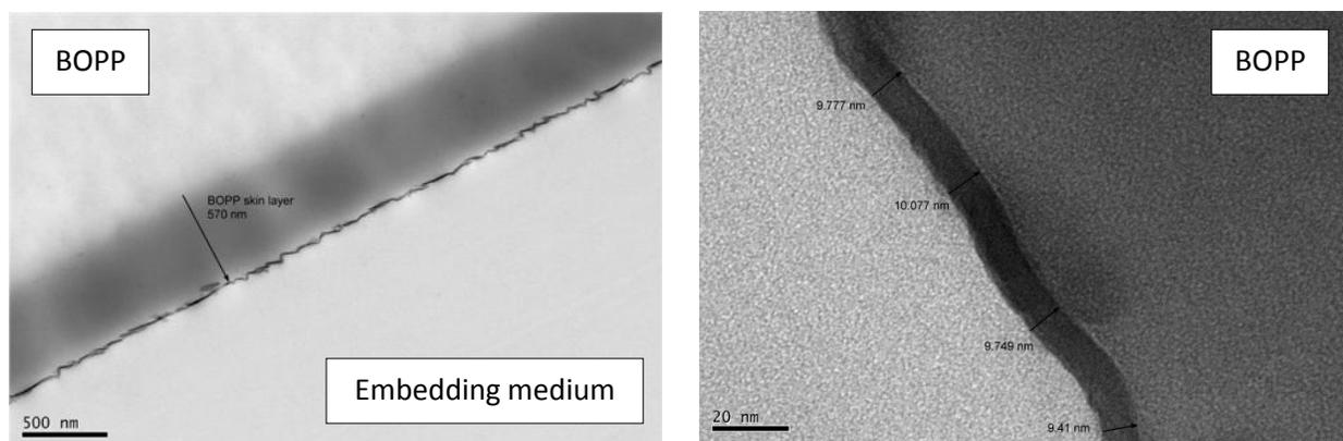
Figure 5 – TEM thickness measurements on  $\text{AlO}_x$  coated BOPP film
