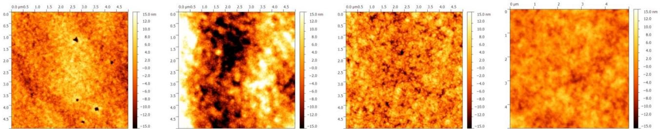
*Figure 4 – 5 x 5  $\mu\text{m}^2$  AFM scans of plain film surfaces – from left to right: BOPP A, BOPP B, BOPP C, BOPP D*
