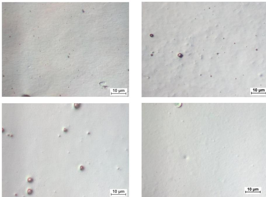
Figure 1 – DIC images of plain film – top left BOPP A, top right BOPP B, bottom left BOPP C, bottom right BOPP D
