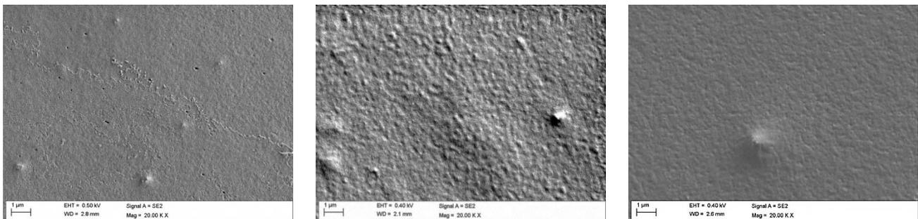
*Figure 3 – SEM images of  $\text{AlO}_x$  coated film surfaces (20 000x magnification) – from left to right: BOPP A, BOPP B, BOPP C*
