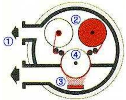
The rolls in a vacuum metallizer must be parallel within a certain tolerance or wrinkles will occur in the metallized plastic film. Wrinkles in the plastic film often result in the product becoming non-recyclable scrap which is costly.
