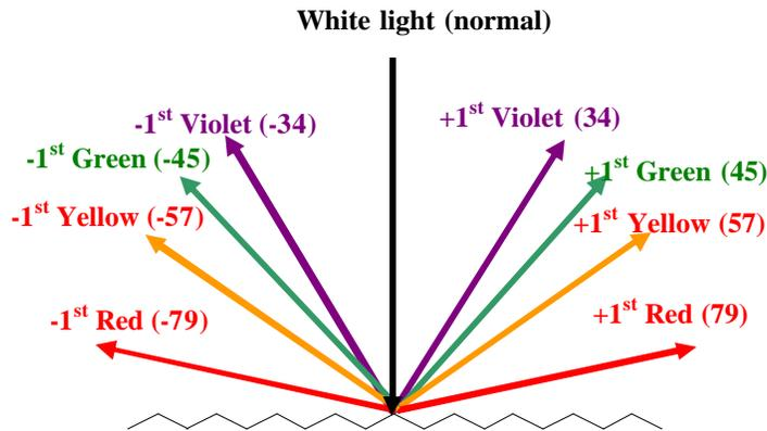
**Figure 1. Spectral distribution of diffractive orders at normal incidence for a 1400 l/mm grating**
