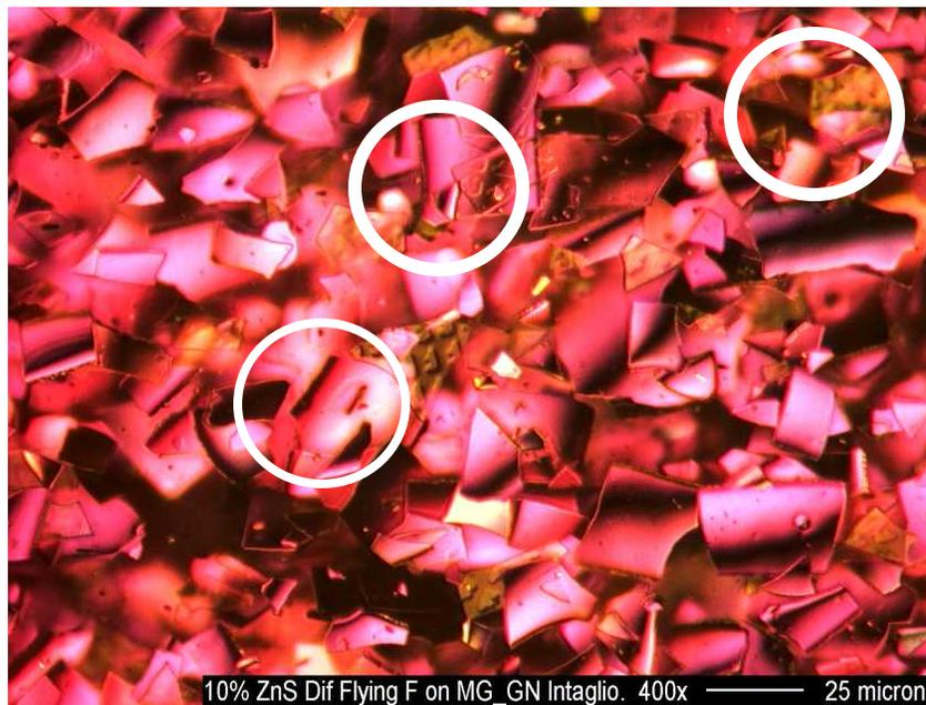
Figure 11. Semitransparent unshaped flakes in Mg-Gr color shifting pigment
