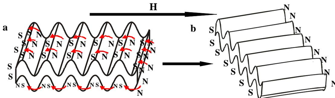
Figure 8. Preferential orientation of a grating particle in the presence of magnetic field H
