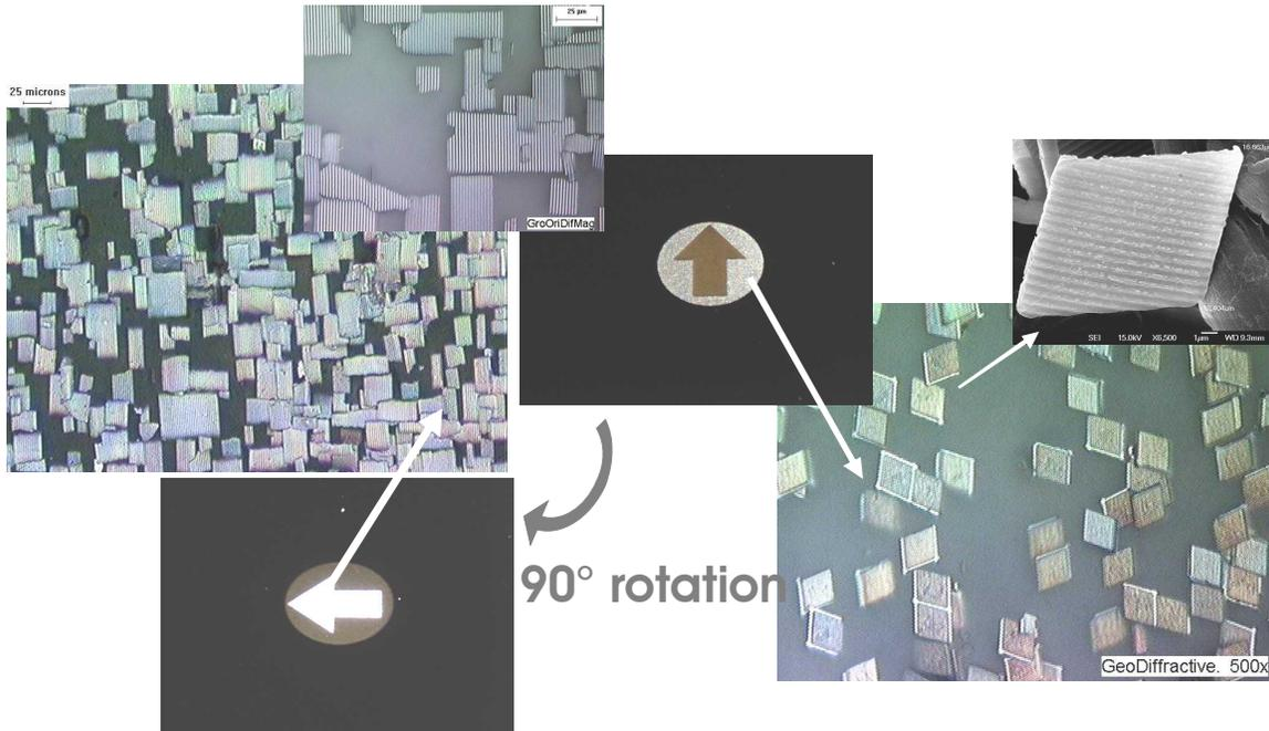
Figure 9. Printed DOVID with the outside circle printed with the grooves oriented  $90^\circ$  with respect to the grooves in the arrow
