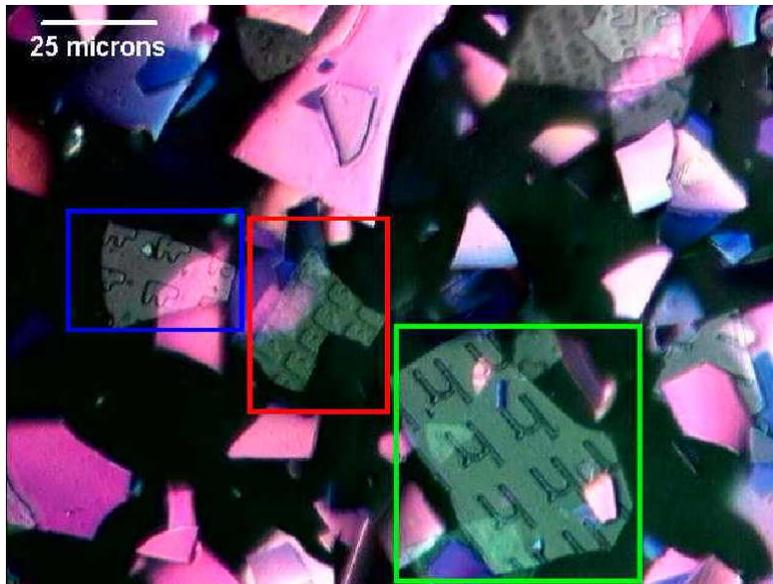
Figure 12. Semitransparent unshaped flakes in BI-Rd color shifting pigment
