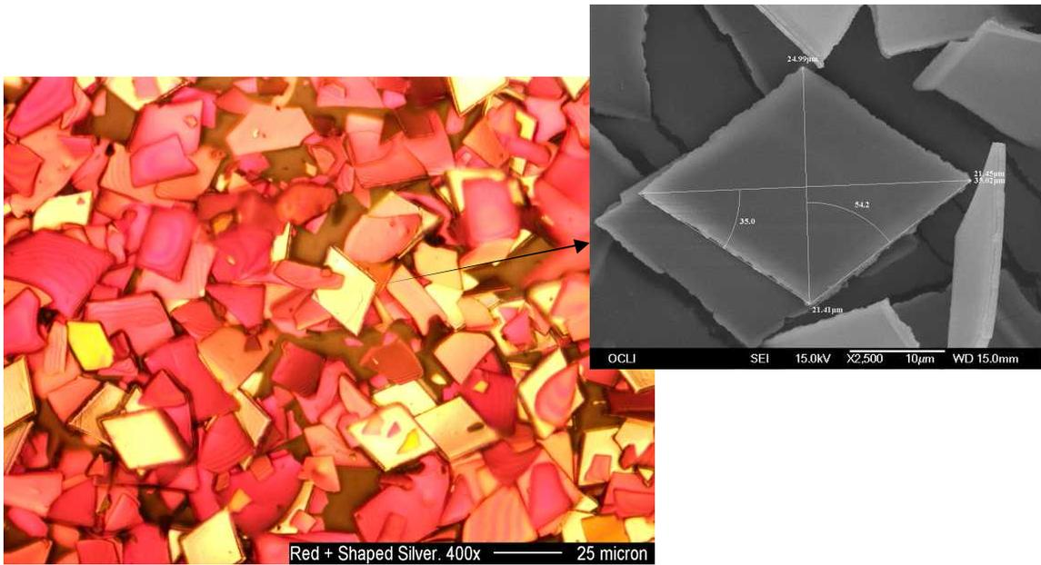
Figure 10. Diamond shaped aluminum flakes in a Red-Gold Color Shifting pigment
