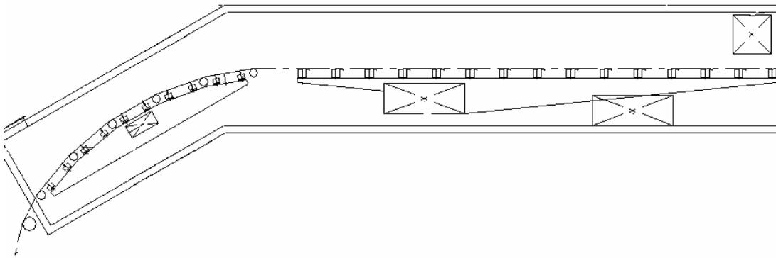
Fig. 5. Quiet zone for controlled evaporation of solvents in thick coatings.
