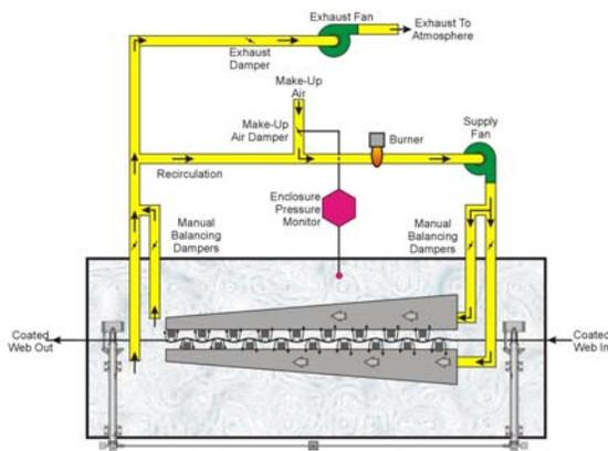
Fig. 2. Tapered air distribution header
