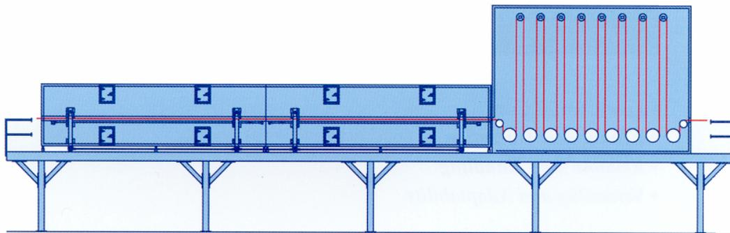
Fig 7. Custom accumulator style dryer used to prevent face roll contact of the coated side of the web.
