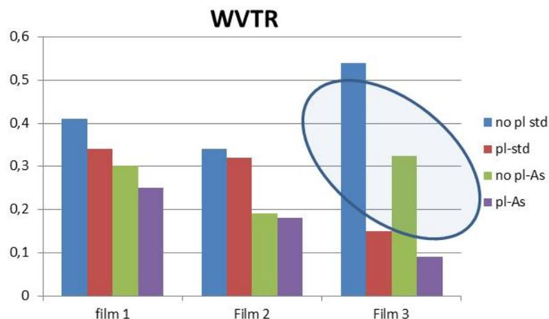
The machine design impact on bopp barrier properties has been studied by comparing barrier results from running same films on three different machines representing nearly 20 years of machine construction technology. Significant technical evolution are relevant to the following areas :
