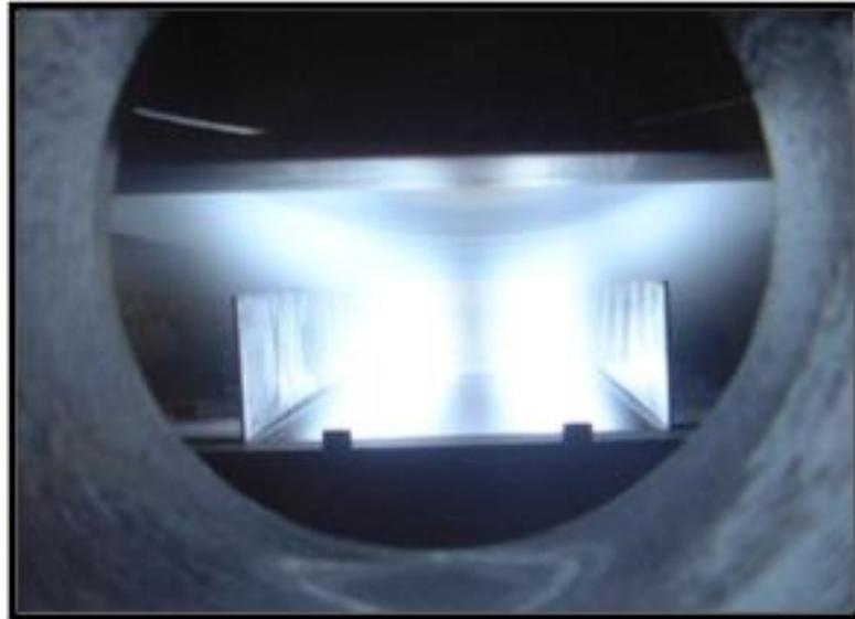
Figure 3. Planar magnetron pre-treatment source.
