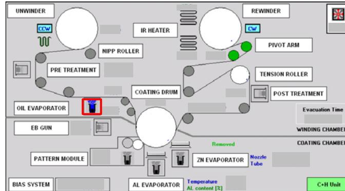
Figure 2: Screen-shot showing the position of the oil evaporator in the winding system of the web coater.
