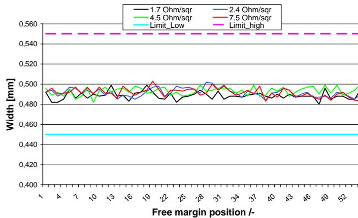
Figure 7: Free margin width distribution across the web for films deposited with different resistivity. Virtually no variation across the web is observed. The specification can be held with a  $c_{pk}$  of 4.88.
