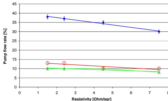
Figure 6: Oil flow rate as a function of metal layer thickness (resistivity), at constant web speed, using different set of nozzles.
