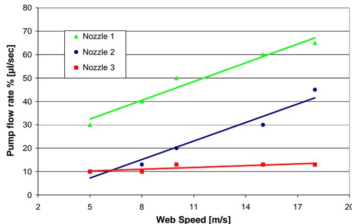
Figure 4: Pump flow rate as a function of coating speed during deposition of  $1.5 \Omega/\text{sqr}$  Al using different nozzles.
