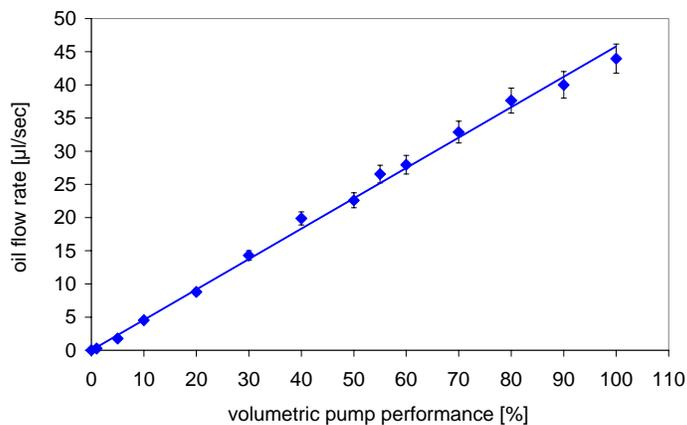
Figure 3: Oil flow rate as a function of pump speed.
