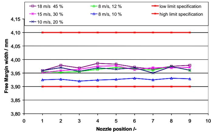
Figure 5: free margin width of “nozzle 2” obtained for different coating process conditions. If the pump rate is adapted properly, the free margin width can be held within tight tolerances. If the pump rate becomes insufficient, the free margin width and edge steepness deteriorates.
