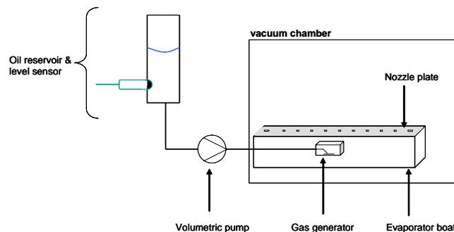
Figure 1: Schematic representation of the flash evaporator. The gas (vapor) generator and main housing are placed in the vacuum winding chamber, while the other units, oil reservoir and volumetric pump are located outside the vacuum chamber.
