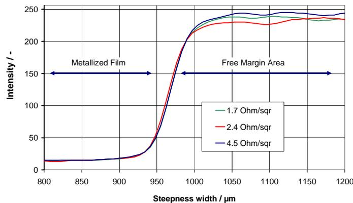
Figure 8: steepness of free margin left edge characterized for different metal layer thickness coated at constant web speed (8 m/s) at optimized pump rate using the “nozzle 2”.
