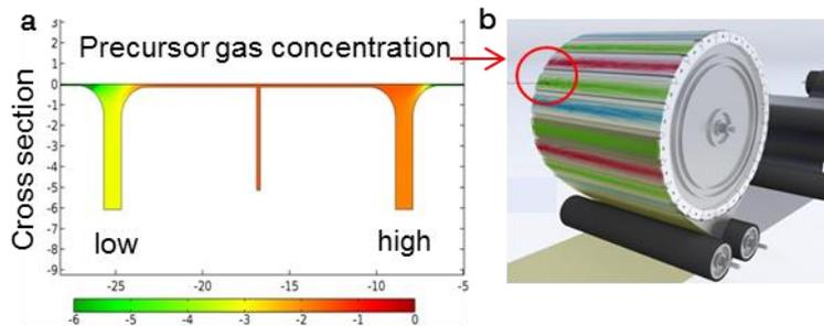
(a)COMSOL simulations of precursor gas flows. (b)Schematic of ALD drum.
