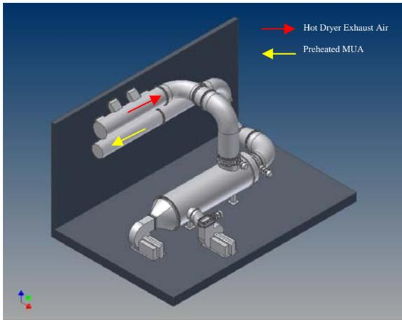
**Fig 5. Energy Recovery from Dryer Exhaust**
