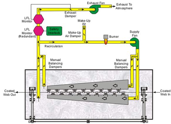
**Fig. 7. LEL Control of Exhaust Volume**
