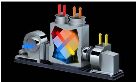
**Cutaway View of Indirect Air-to-Air Heat Exchanger**
