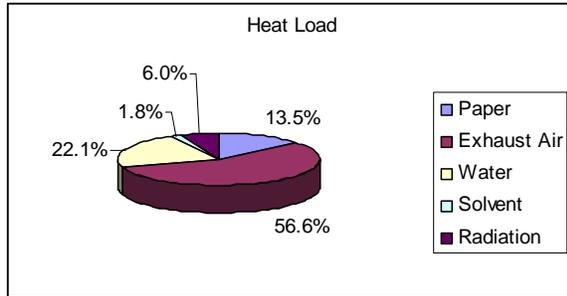
**Fig. 4 – Heat Load Value Map (based on heat set printing application)**
