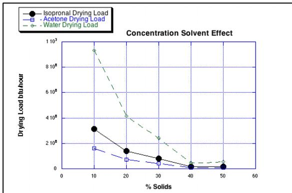
Fig. 9 – Effects of Solvent Concentration on Drying Load
