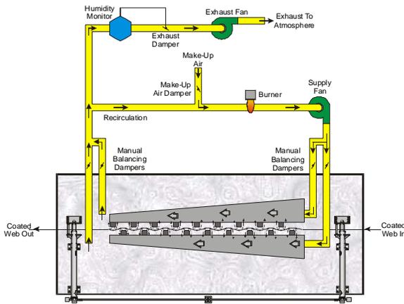
**Fig. 6 – Humidity Control of Exhaust Volume**
