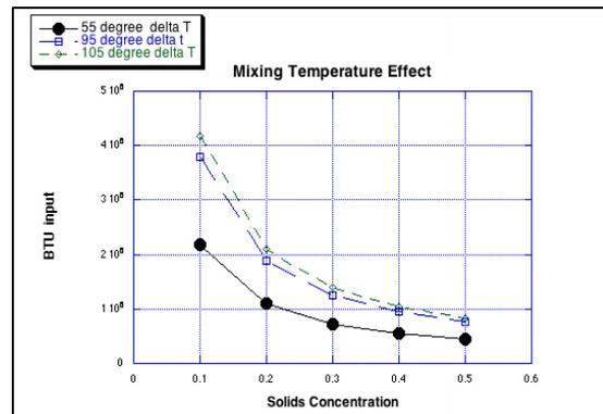
Fig. 12 – Mixing Temperature in Relation to Solution Concentration
