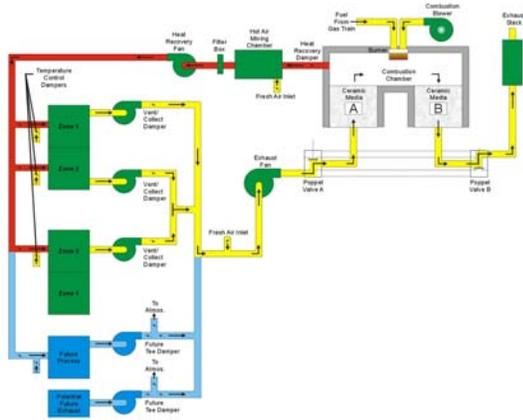
**Direct Air Heat Recovery – Combustion chamber air mixed is with fresh air and returned to process**
