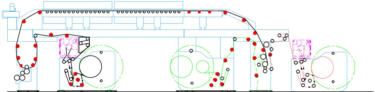
*Nordmeccanica Duplex Combi machine: in red the rollers which can be advantageously replaced with carbon rollers.*
