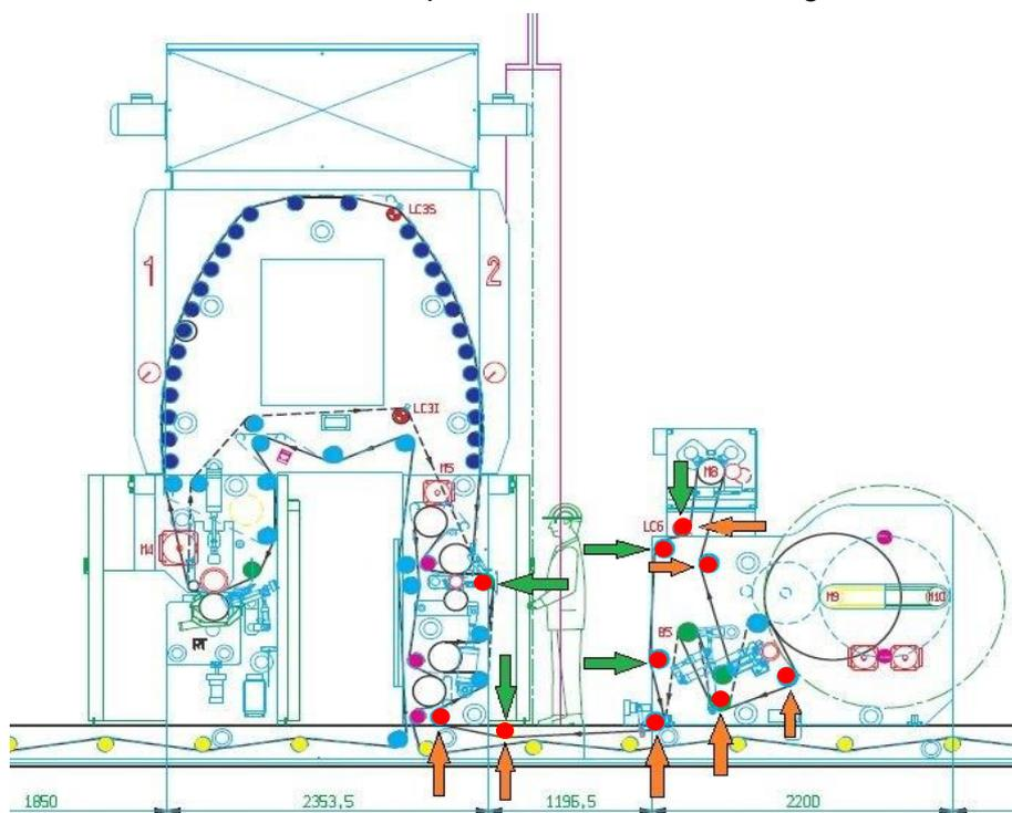
evaluate the possibility to reduce the bearing size (as explained before) replacing also the inner shaft with a smaller one.
