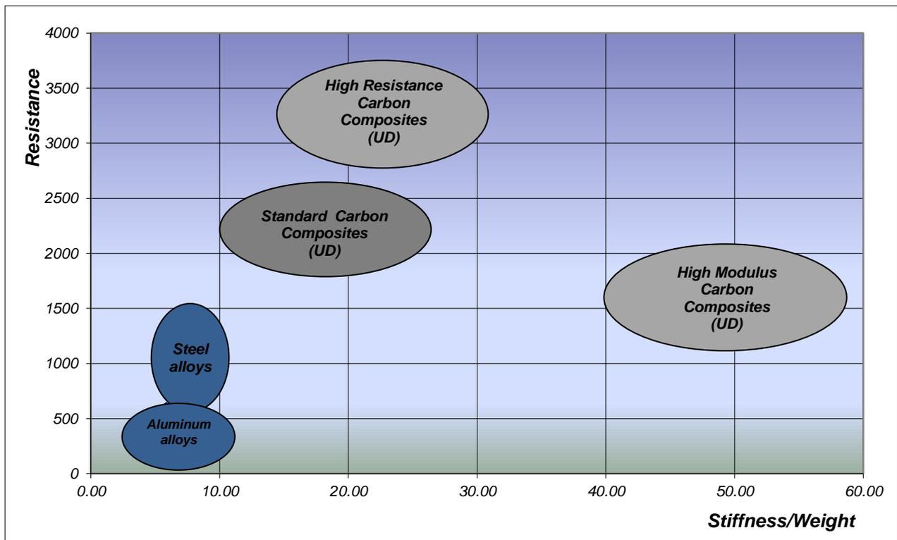
A high performance carbon fiber composite is usually composed by an epoxy matrix reinforced with many different types of carbon fibers depending from the performance requests of the component.
