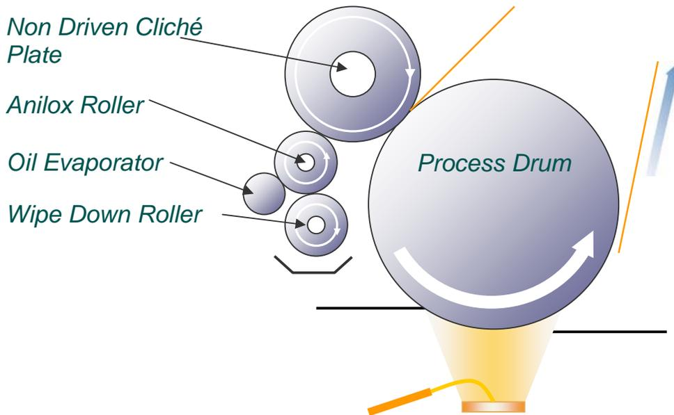
**Figure: 3.0 A simplified schematic to illustrate a pattern printing system**
