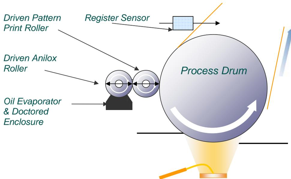
**Figure: 4.0 A simplified schematic to illustrate a pattern printing system with registration capabilities**
