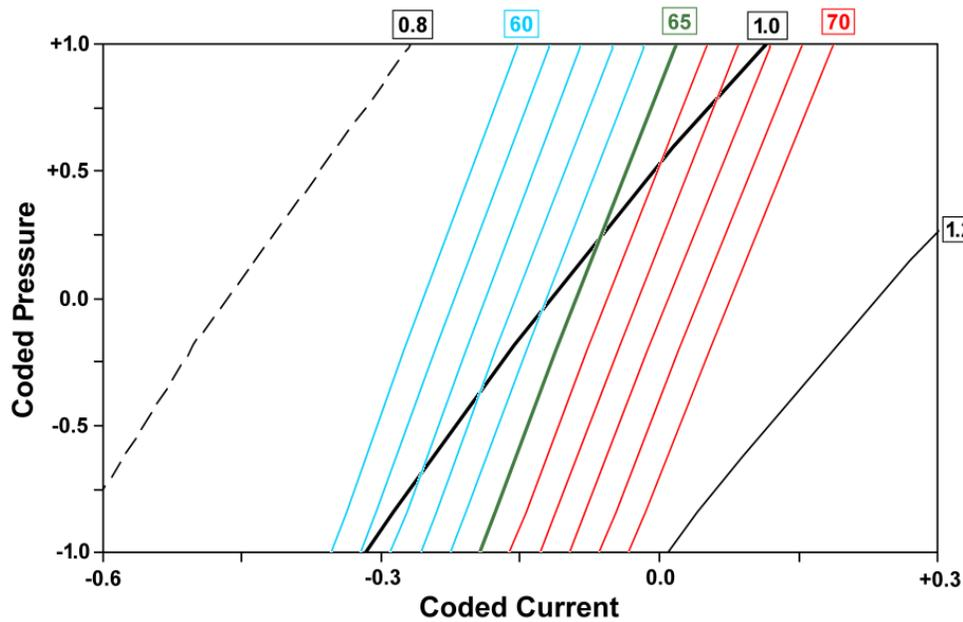
**Figure 5.** Contour plot from analysis of the results from the factorial experiment. Black contour lines show constant deposition rate. Coloured contour lines show constant heat flux: blue contours show heat flux lower than that of the green contour, while red contours show higher heat flux.
