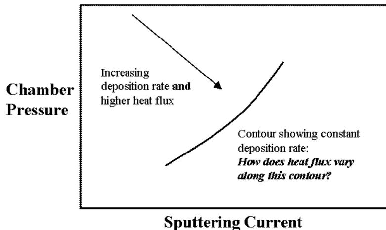
**Figure 3.** Illustration of the relevant aspects of the representative 2-D model under discussion.
