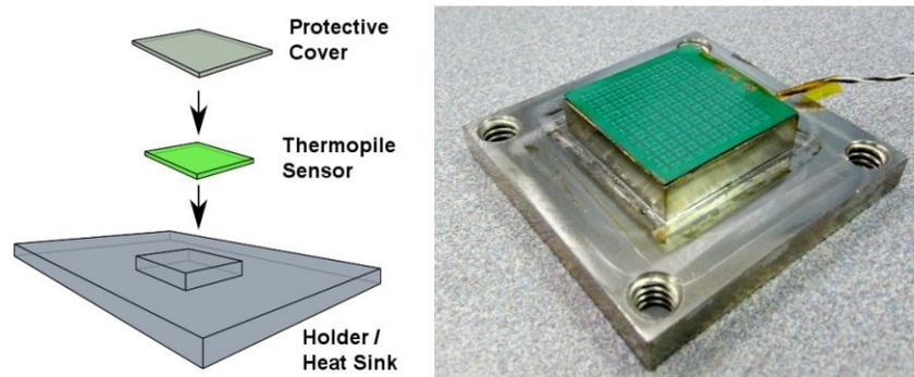
**Figure 2.** Heat flux sensor. The drawing on the left shows an exploded diagram of the components. The image on the right shows the assembled sensor without the protective cover.
