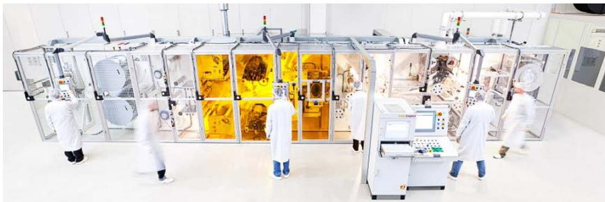
*Figure 1a: roll-to-roll encapsulation tool*
