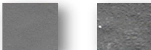
**Fig. 3 Atmospheric plasma micro-etching effect of PE film, 30,000 SEM magnification**
