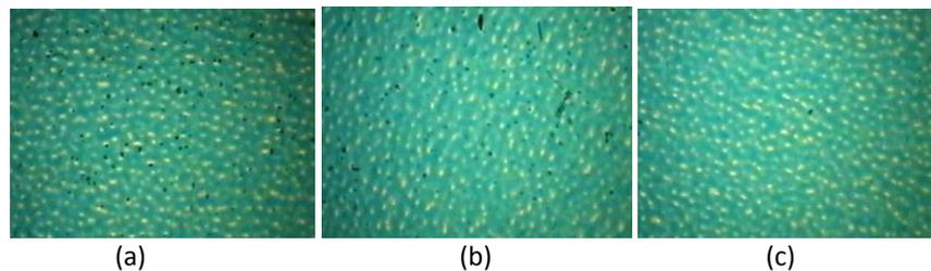
**Fig. 4 Micrograph of PET film (a) untreated with low molecular weight organic contamination, (b) after corona discharge cleaning, and (c) after oxygen-based atmospheric plasma cleaning.**
