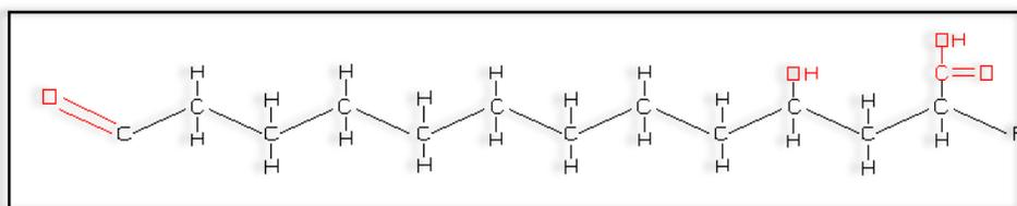
**Fig.2 Plasma activation of polymer surface by creation of free radicals through substitution.**
