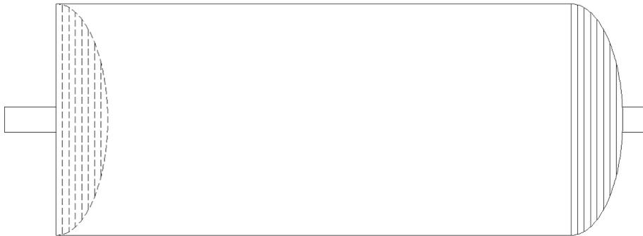
When the coating shows thickness variations in the machine direction, it interferes with tension control during winding, and may result in starring. In the diagram below, looking at the end of a wound roll, starring is shown as the poorly wound layers in the middle of the roll.
