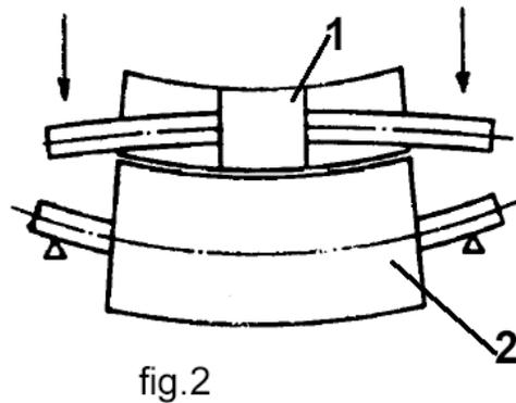
In our recommended (patented) design, the nip roll has deflection compensation built-in. This results in the nip loading forces being applied more in the center of the roll, producing a very uniform nip gap and therefore more uniform coating coverage.
