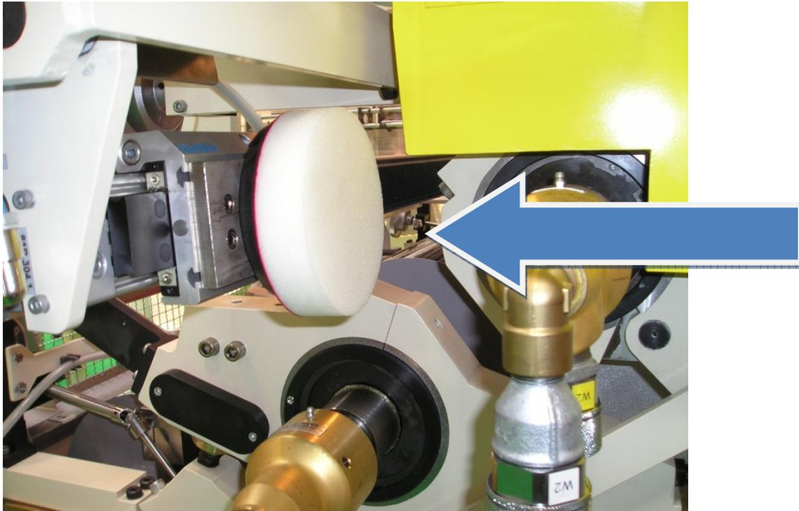
Dust can be removed from the web by installing a commercially available web cleaner like the one shown below.
