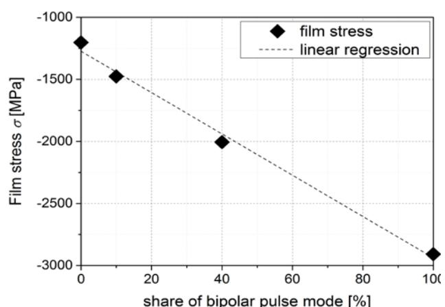
Figure 1: Adaption of film stress of AlN layers (thickness: 500 nm) with the unipolar/bipolar hybrid pulse mode.
