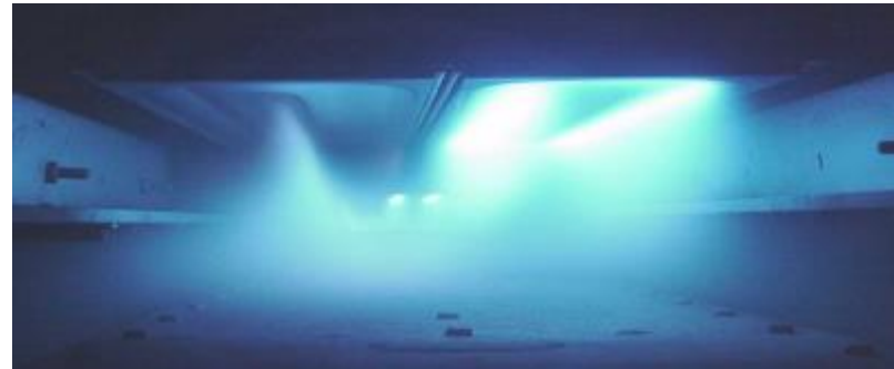
Discharge during the two phases of the bipolar pulse
