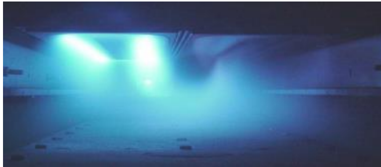
Discharge during the two phases of the bipolar pulse
