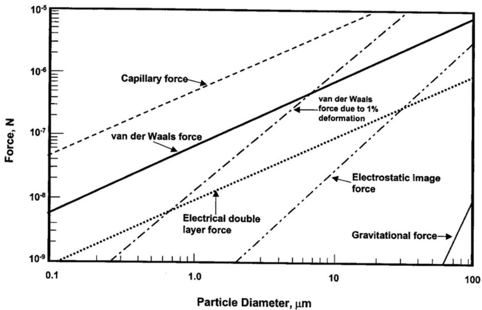
The adhesion forces are shown as a function of the diameter for an  $\text{Al}_2\text{O}_3$  particle on a Si substrate [20-21, 37].
