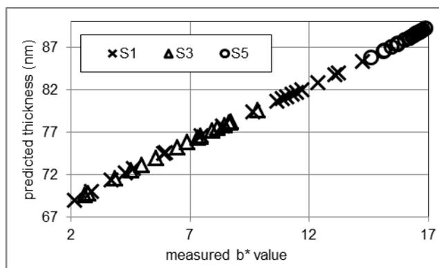
Fig. 2 Thickness results based on  $b^*$  measurements
