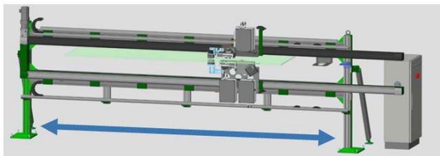
Fig. 4 Traversing measurement system, the arrow indicates the moving range of the measurement probes
