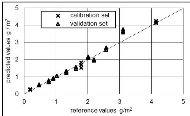
Fig. 3 Plot of the predicted grammage values for three calibration samples and 10 validation samples
