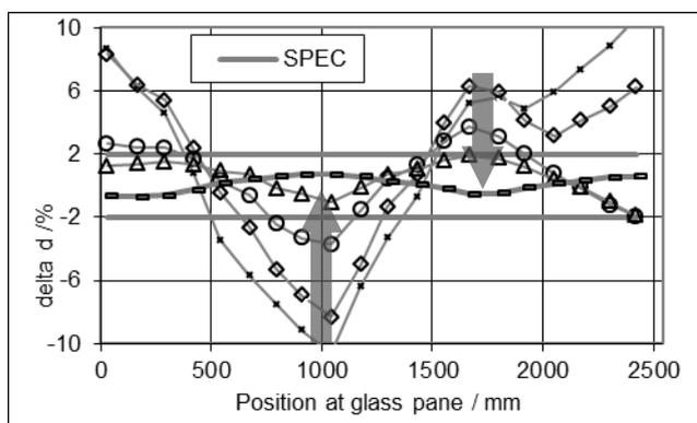
Fig. 5 Example of a cross section plots of coating thickness variation ( $d/\%$  of nominal value) for process monitoring (six different glass panes)
