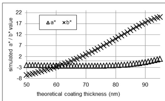
Fig. 1 Correlation of  $a^* / b^*$  and coating thickness of ZnO calculated with the SCOUT modelling software.
