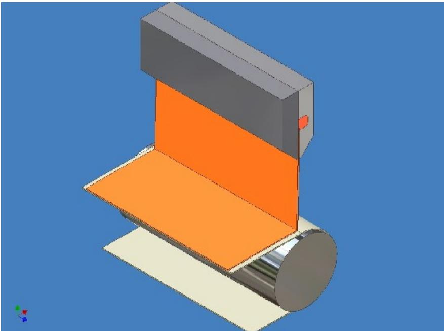
Figure 1. Curtain coating with a slot-curtain die
