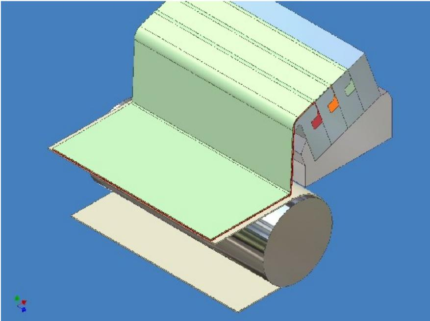
Figure 2. Curtain coating with a multilayer slide-curtain die (Cutaway view displays slide format die with three manifold plates.)
