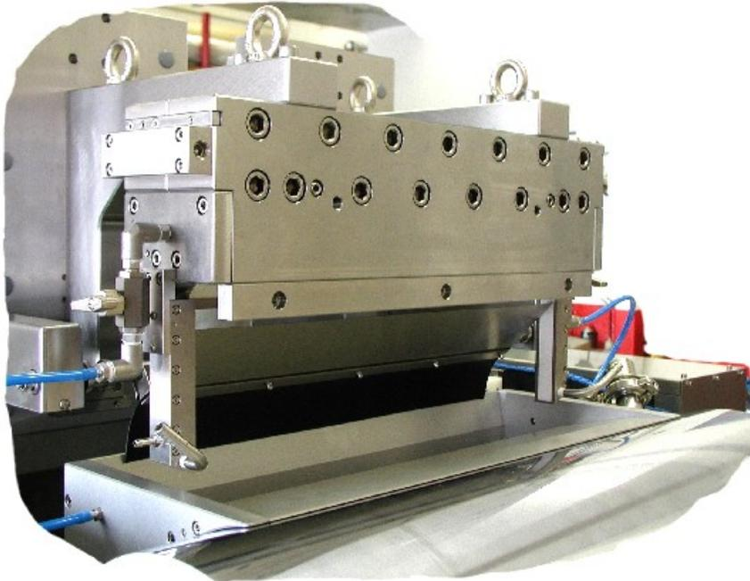
Figure 3. Slot-curtain die equipped for commercial production
