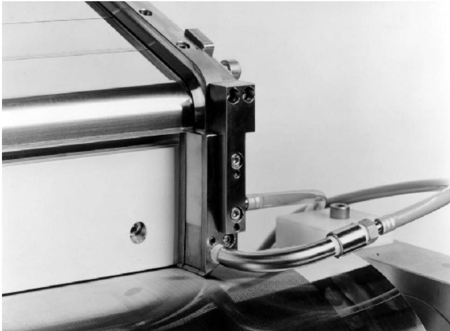
Figure 4. TSE proprietary curtain edge guide system utilizing lubricating edge flow
