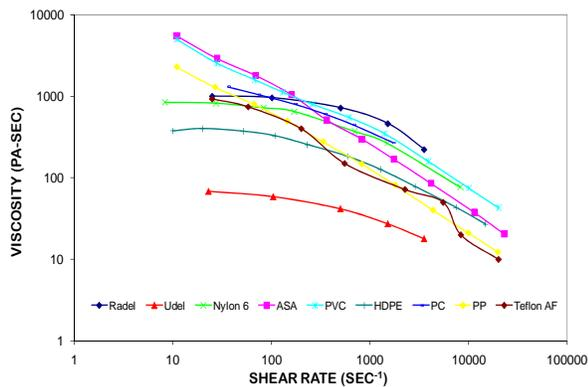
Figure 3. Viscosity versus Shear Rate - Polymers
