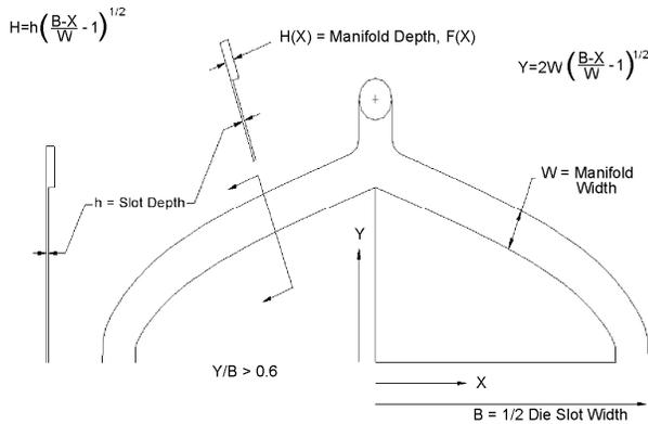
Figure 4. Constant Shear Manifold Design Equations
