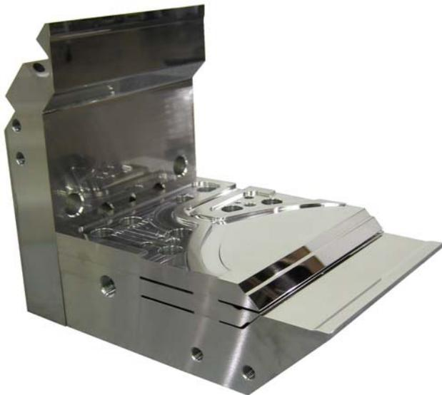
Figure 7. Eight Inch Wide Triple Manifold Design
