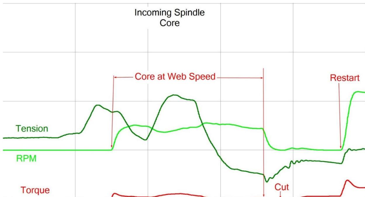
The next chart shows how feed-forward techniques can be implemented. Torque is adjusted up or down at different parts of the index cycle to account for web length changes and other disturbances. The feed-forward techniques can be based on models of tension during the index or empirically based on tension
