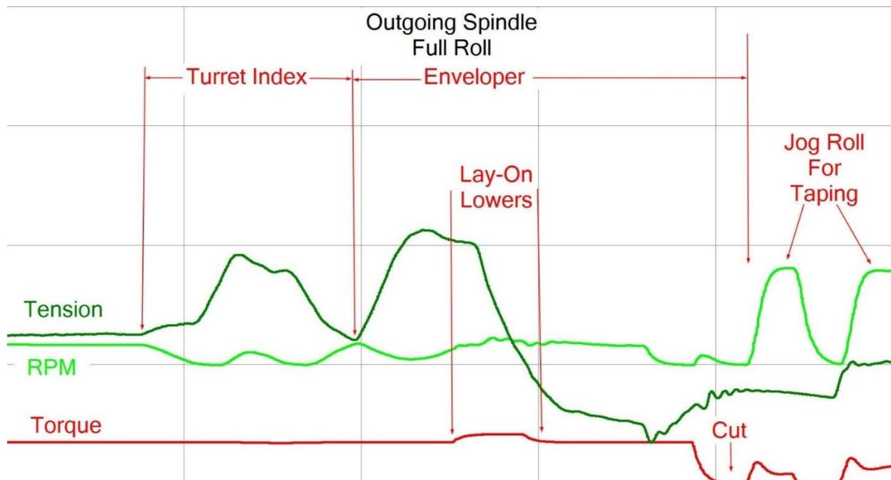
The chart below shows tension and torque for the incoming core for the same index. The incoming core is run to web speed with a speed regulator. We see torque vary as the turret moves and the lay-on roller lowers. After the cut, the web is attached to the core and the core is accelerated to an overspeed before settling into its steady running under tension control.
