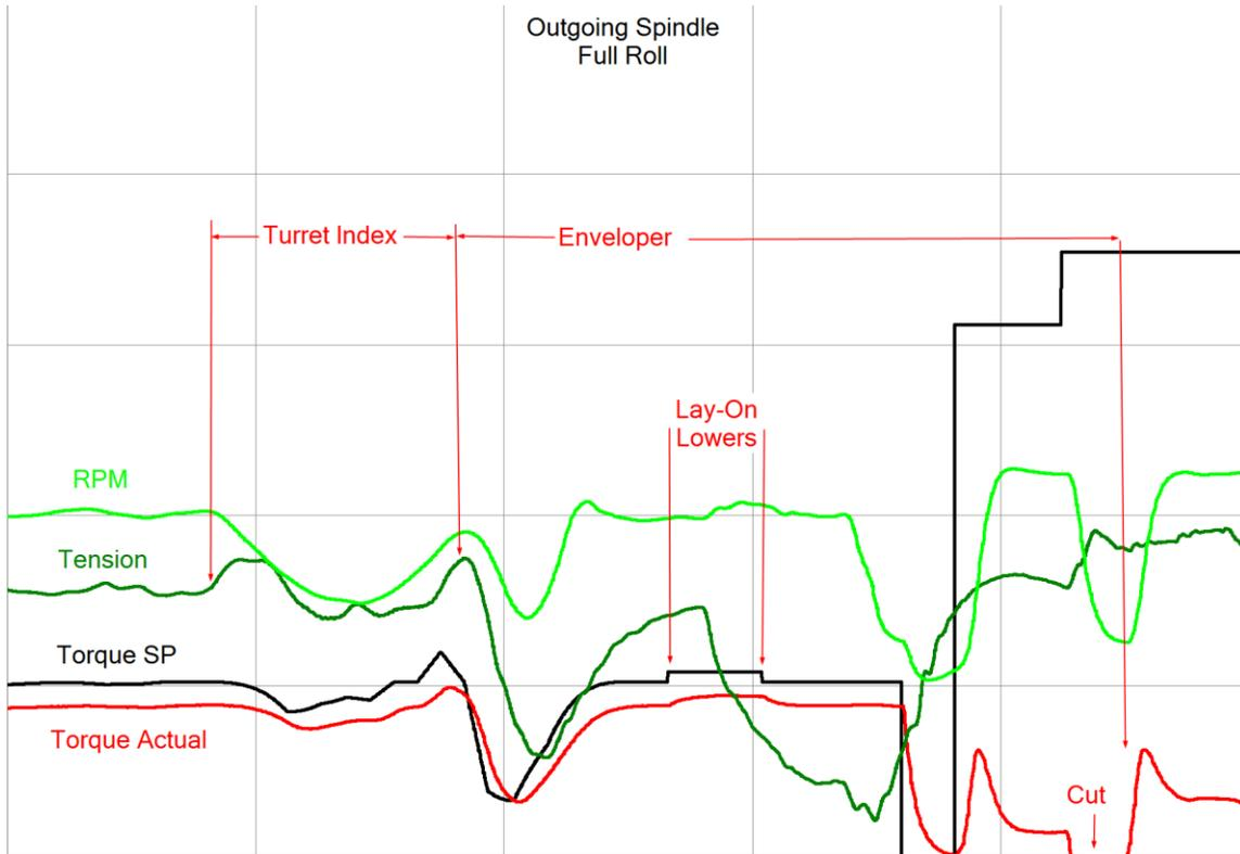
In this case, the spindle control was by tension through the torque regulator. In the case of spindle control using tension through the speed regulator we note that the tension regulator is often disabled by torque hold or torque memorize during the turret index. Some spindle drives remain in speed control during the index and feed-forward techniques are available to modify the spindle RPM during the index to hold tension to acceptable values.
