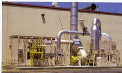
Concentrators reduce the air volume being sent to an oxidizer, increasing the capacity and efficiency of an existing oxidizer system. Large air volumes with low VOC concentrations are absorbed into a concentrator then desorbed in a condensed, smaller volume before being sent to the oxidizer.
