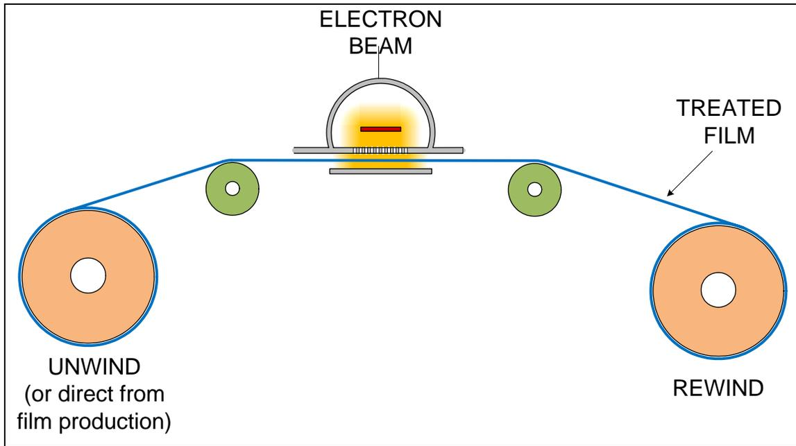
Figure 2. Film Crosslinking
