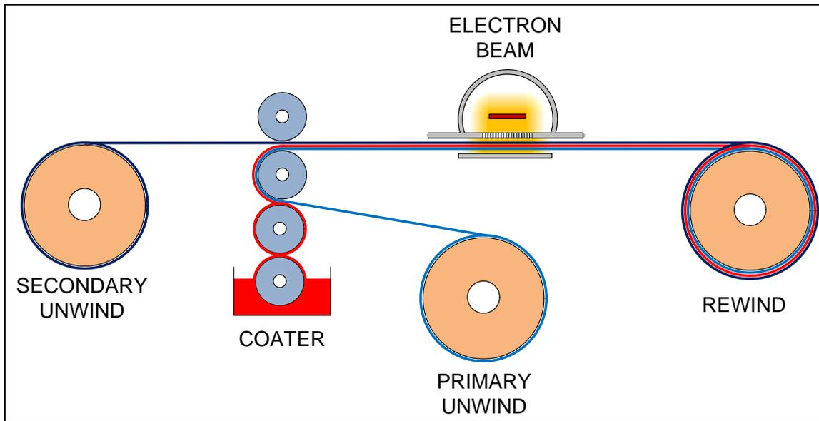
Figure 5. Adhesive Laminating
