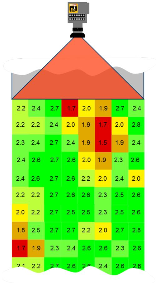
Example for an inline-evaluation of the optical density for a metal coated packaging film.
