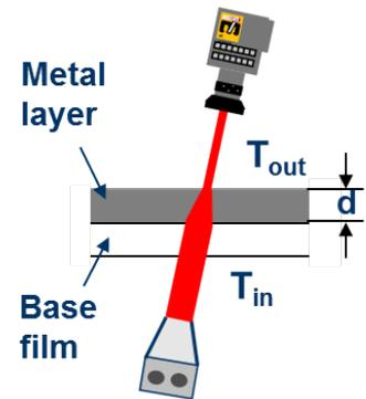
Fig. 4: Monitoring of coating thickness (i.e. optical density) of metal layers
