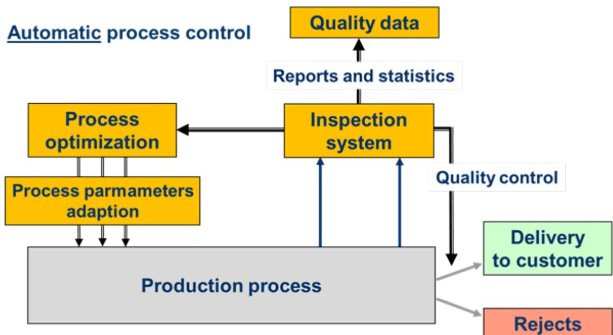
Fig. 2: Automatic process control of a production process by AOI data
