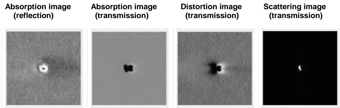
Fig. 1: Multiple Image Defect Analysis (MIDA) of the same defect (inclusion in plastic film)
