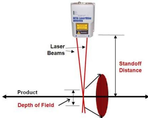
**Figure 15. Non-contact gauge uses a dual-beam laser technology to measure product velocity and length**
