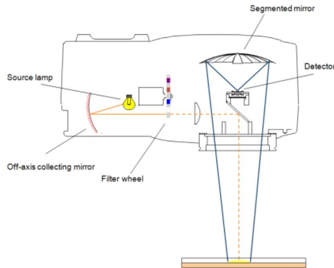
**Figure 6. IR backscatter gauge schematic. IR light source is focused onto a spinning filter wheel that allows pulses of light through at specific wavelengths. These light pulses interact with the web, where the energy is preferentially absorbed. The detector converts the remaining light energy to a useable signal for data processing.**
