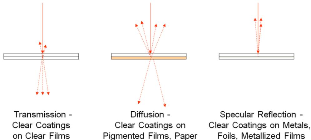
**Figure 7. Types of IR energy behavior on substrates**
