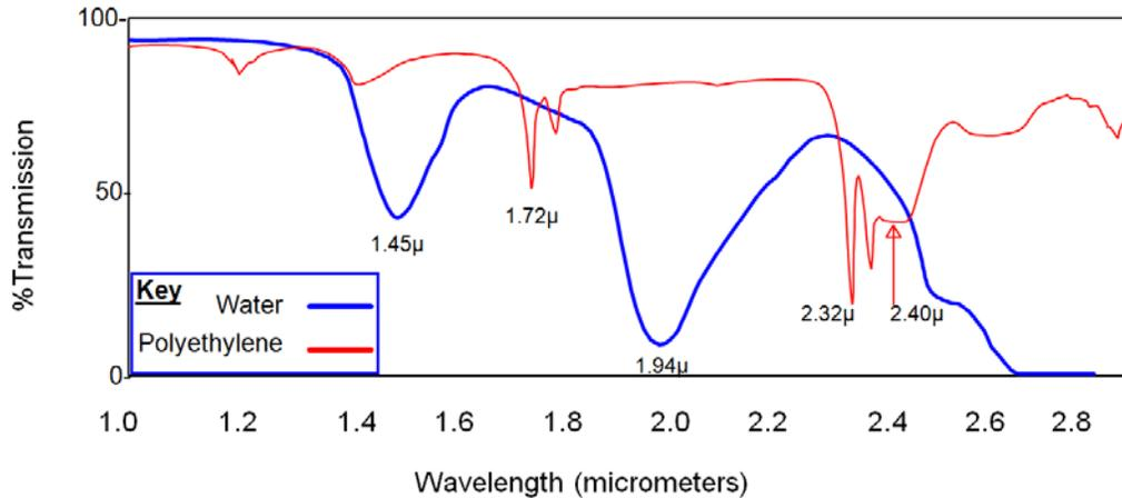
**Figure 5. A single infrared sensor can measure both the PE substrate thickness and the water-based coating weight**
