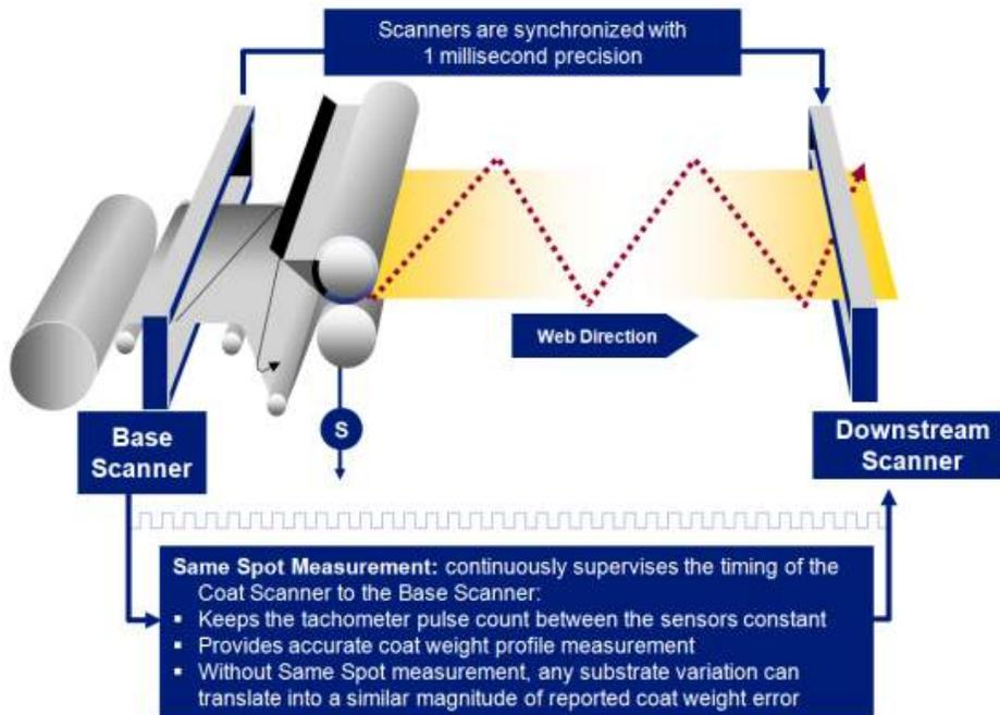
**Figure 13 – Same Spot Measurement logic**
