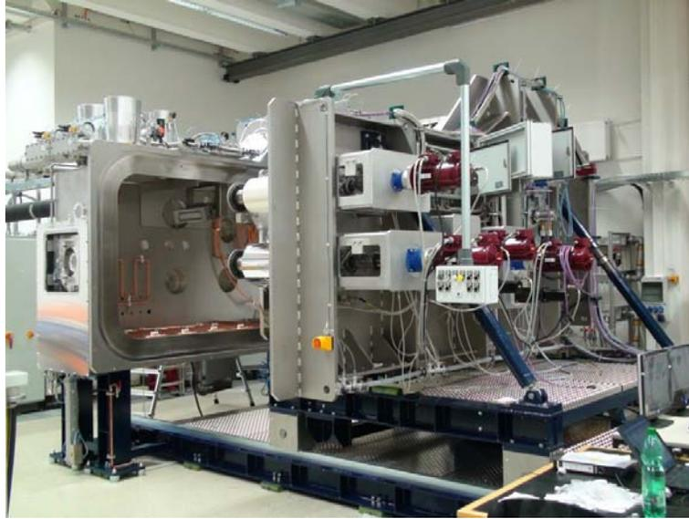
**Figure 6.** A photograph of the roll-to-roll coater with the open process chamber.
