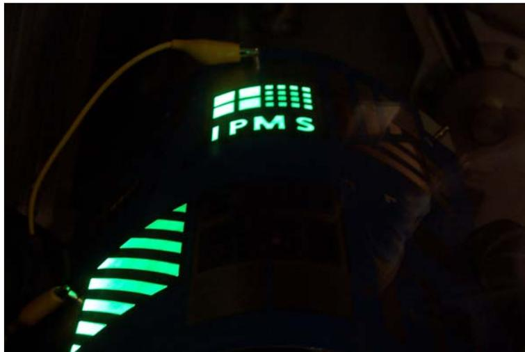
**Figure 1.** The photograph shows a green OLED deposited aluminum sheet under electrical testing. Power efficiencies between 20 - 25 lm/W is well possible for green *pin* OLED stacks on aluminum sheets (for comparison: A 75 W filament lamp has  $\approx$  12 lm/W).
