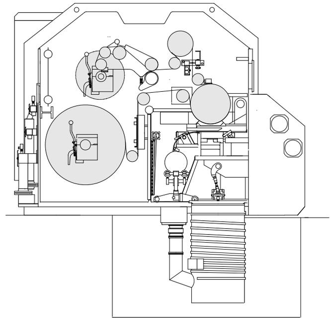
Figure 1: Schematic view of modern web Metallizer for aluminum on films, courtesy of Applied Films
