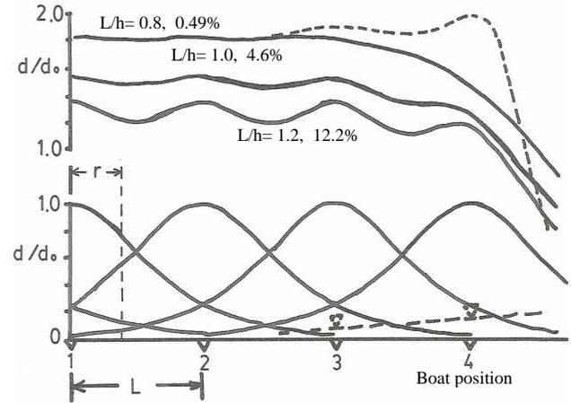
Figure 4: Figure 4 of reference 4, Schematic diagram of continuous metal layer formed from overlap of deposit from each boat
