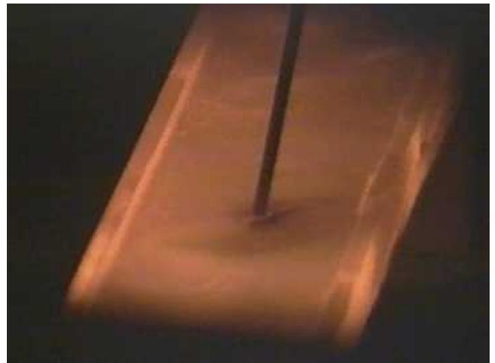
Figure 2: Aluminum wire melting and evaporating on a resistance heated ceramic metallization boat, courtesy of Applied Films
