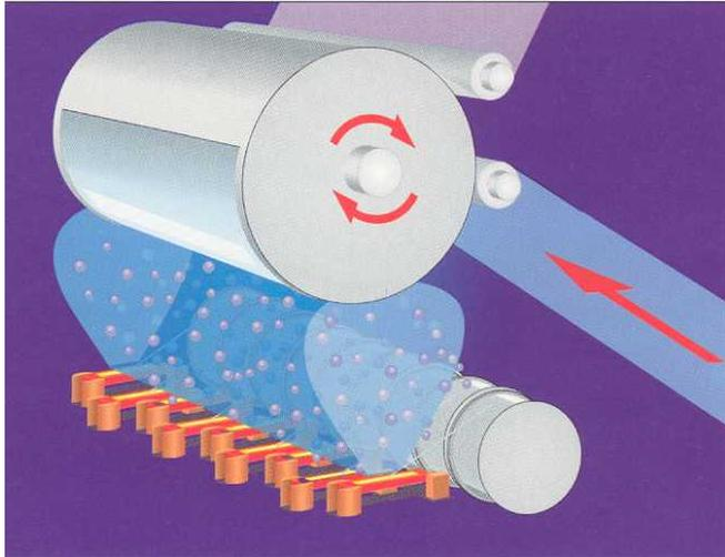
Figure 3: Schematic diagram of metallization process showing evaporation from a series of boats to produce a continuous Aluminum film coating, courtesy of Applied Films
