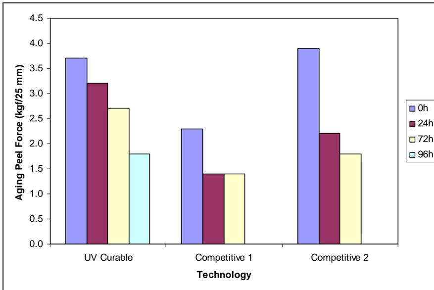
**Figure 12. Resistance to Aging at 80°C & 85% RH**
