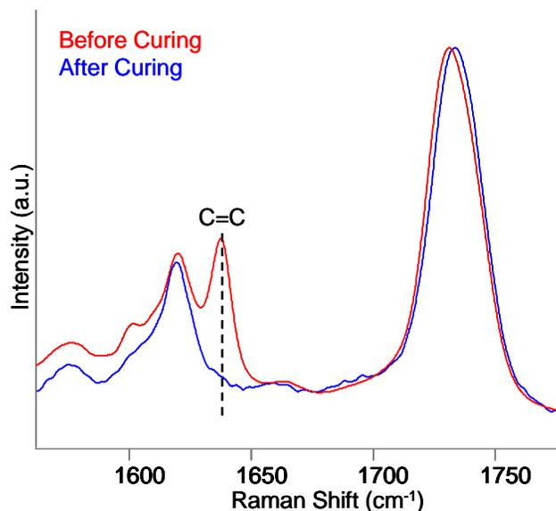
**Figure 8. Confocal Raman Microscopy of UV PSA Coatings (1 mil)**
