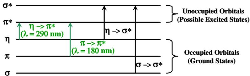
**Figure 3. Electronic Excitation of C=O in Acrylate**
