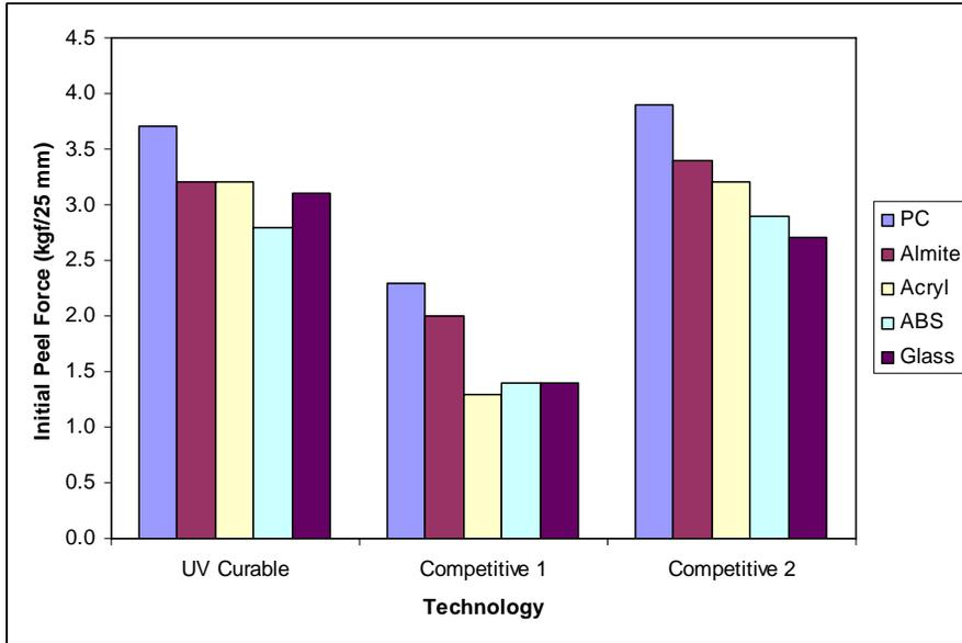
**Figure 11. Peel Adhesion on Various Substrates**
