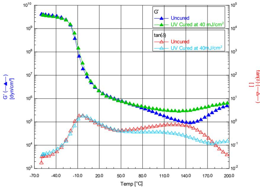
**Figure 10. Temperature Dependence of  $G'$  and  $\tan(\delta)$  for PSA**
