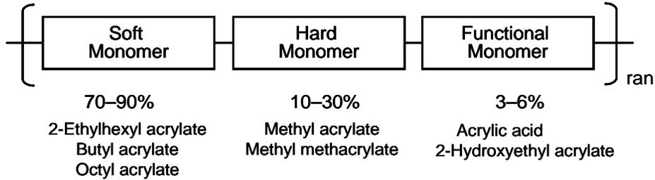
**Figure 2. Typical Acrylic PSA Polymer Composition**
