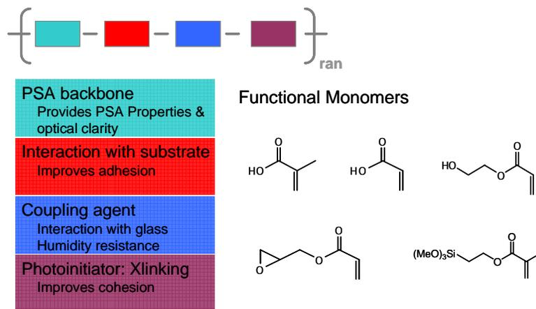
**Figure 7. UV Curable Acrylic Polymer Design and Functional Groups**
