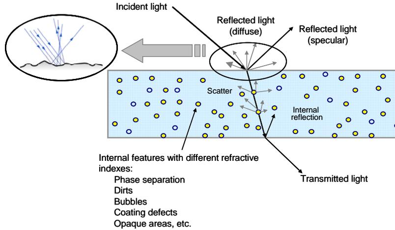
**Figure 4. Coating Quality Impact on Optical Clarity of Coatings**
