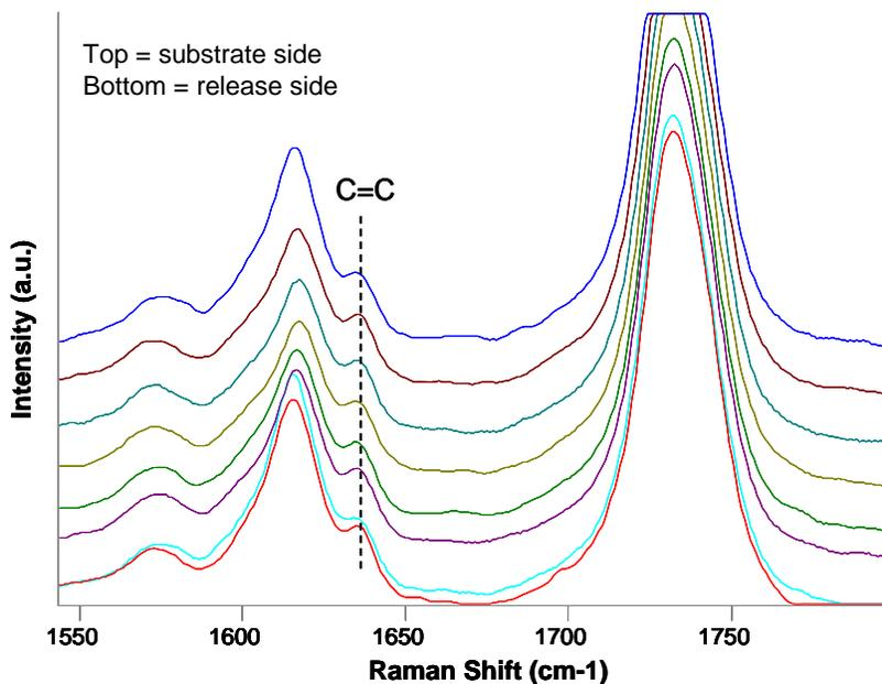
**Figure 9. Confocal Raman Microscopy Map through UV curable acrylic PSA (1 mil) Cured at  $43 \text{ mJ/cm}^2$**
