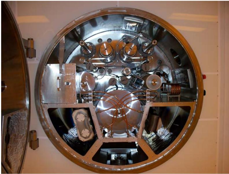
Figure 1: Clean room view of GVE tool vacuum chamber showing (bottom half) three independently pumped process zones.
