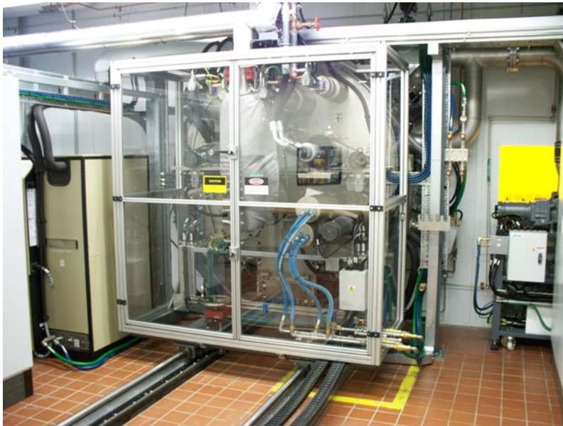
Figure 2: Service core side of GVE tool showing winding mechanism (top). The plasma pre-process zone and dual rotating cathode are shown clockwise on the right hand side.
