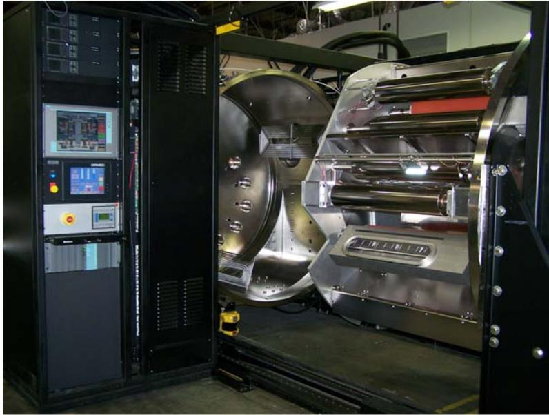
Figure 3: CHA Industries Mark 80 roll coater with web winding and process zones mounted on the front door. The entire assembly moves on floor mounted rails into the vacuum chamber.
