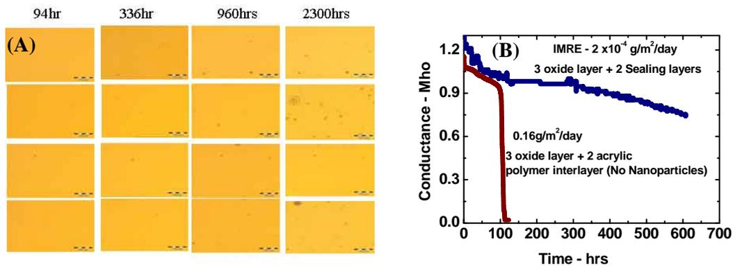
**Figure 2** (A) Microscopic images of calcium sensor at different time intervals at 60°C and 90% RH; (B) Water vapor transport rates for conventional and nanoparticulate barrier stacks
