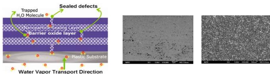
**Figure 1.** IMRE’s barrier substrate technology ‘plugs the gaps’ in technology – (A) Conceptual Barrier Stack, (B) SEM picture (x 10K) of Barrier oxide with pinholes, (C) SEM image (x10K) of defects sealed- barrier oxide film
