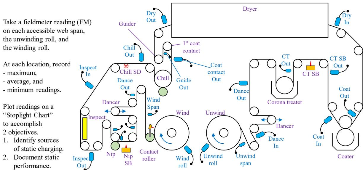
Figure 3.3: Advice for identifying static charging sources and documenting static performance.
