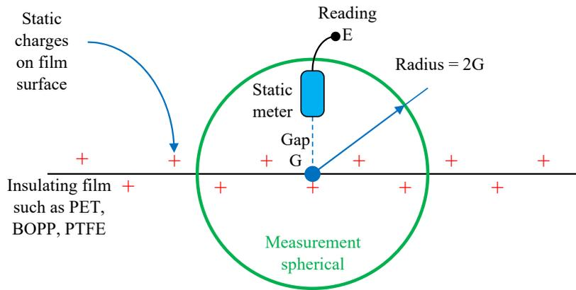
In your “mind’s eye,” draw a dot the web below the fieldmeter. The dot becomes the center of a sphere that expands to a radius of 2G. For reliable readings, the “measurement sphere” must be empty (except for the meter and your hand).
