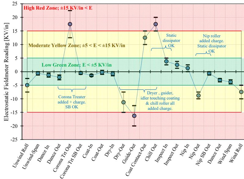
Figure 3.4: Plot fieldmeter measurements to identify charging sources and document static performance.
