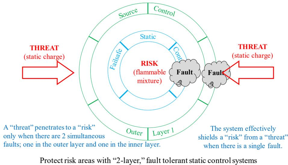
Figure 3.1: Engineering strategy to achieve fault-tolerant static control.
