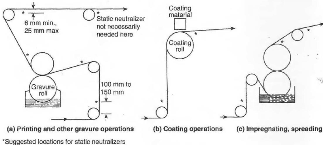
**FIGURE 17.5.3.2.3 Typical Locations for Static Neutralizers.**
