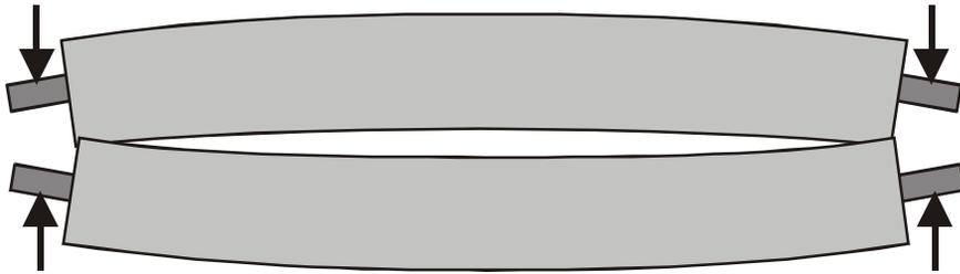
**Figure 2 – Roller Thin Wall Shell Deflection**
