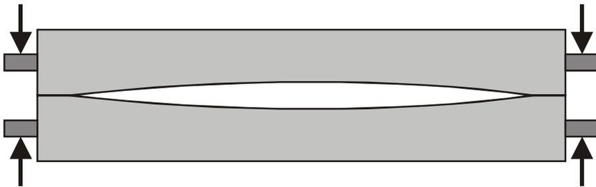
**Figure 3 – Cylindricity Error**
