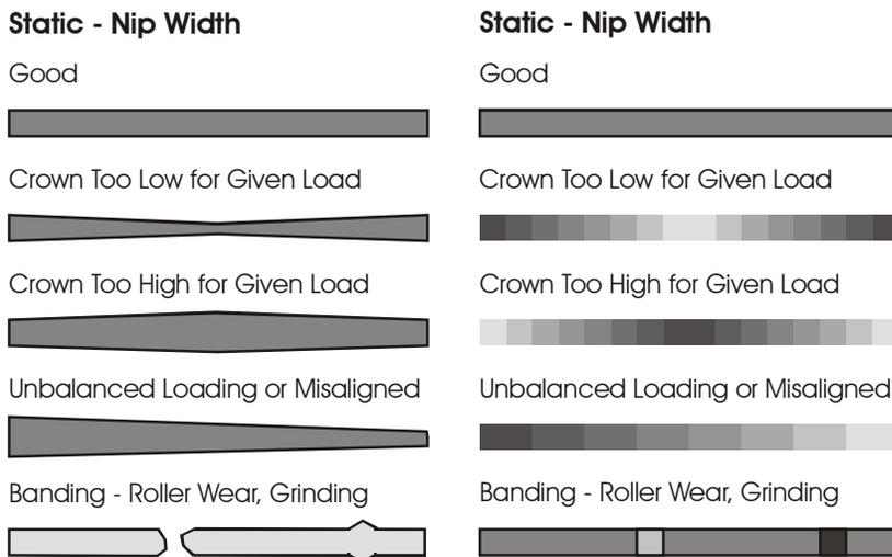
**Figure 8 – Crown Errors**
