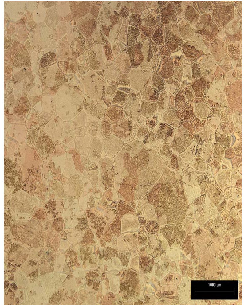
Cast CuGa 25 at% @ 25x
