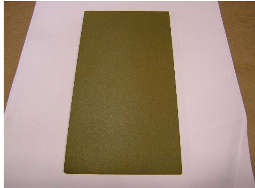
After Machining, CdS PVD Tile
