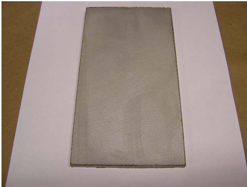
As Pressed CdS PVD Tile (w/redux)
