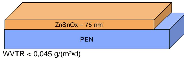
**Figure 8:** Single ZnSnOx layer, deposited by sputtering (substrate 75 μm PEN, WVTR measured at 38°C and 90% r.h.)
