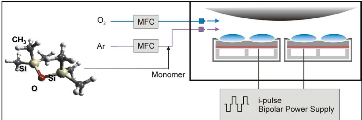
Figure 2: Concept of the magnetron PECVD process
