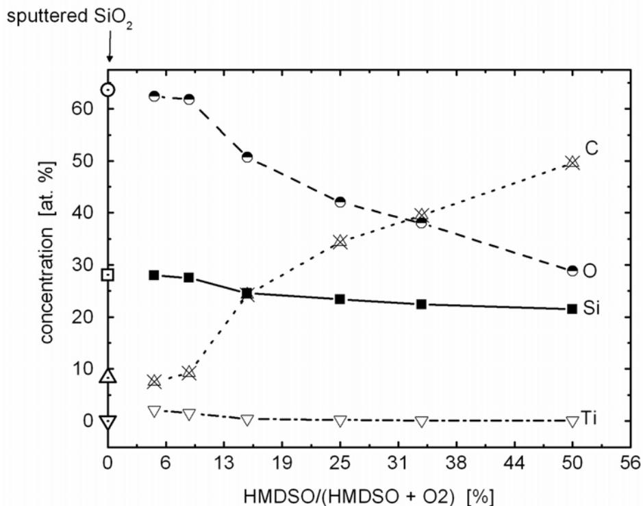
**Figure 5:** Composition of SiO<sub>x</sub>C<sub>y</sub>-layers in dependency on the gas flow of HMDSO and O<sub>2</sub> (layer composition determined by XPS).
