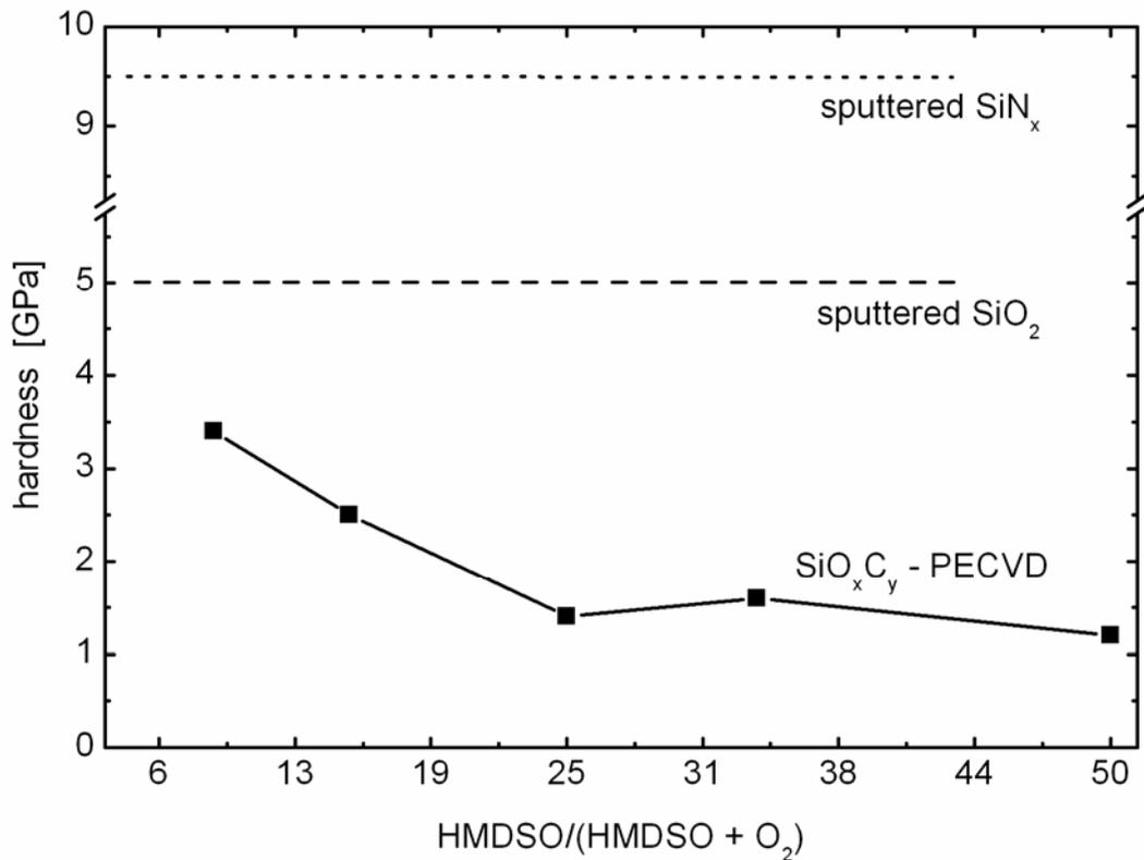
**Figure 6:** Nanohardness of SiO<sub>x</sub>C<sub>y</sub> layers in dependency on the gas flow of HMDSO and O<sub>2</sub> (substrate PET, as reference, the typical hardness of SiN<sub>x</sub> and SiO<sub>2</sub> layers is shown)
