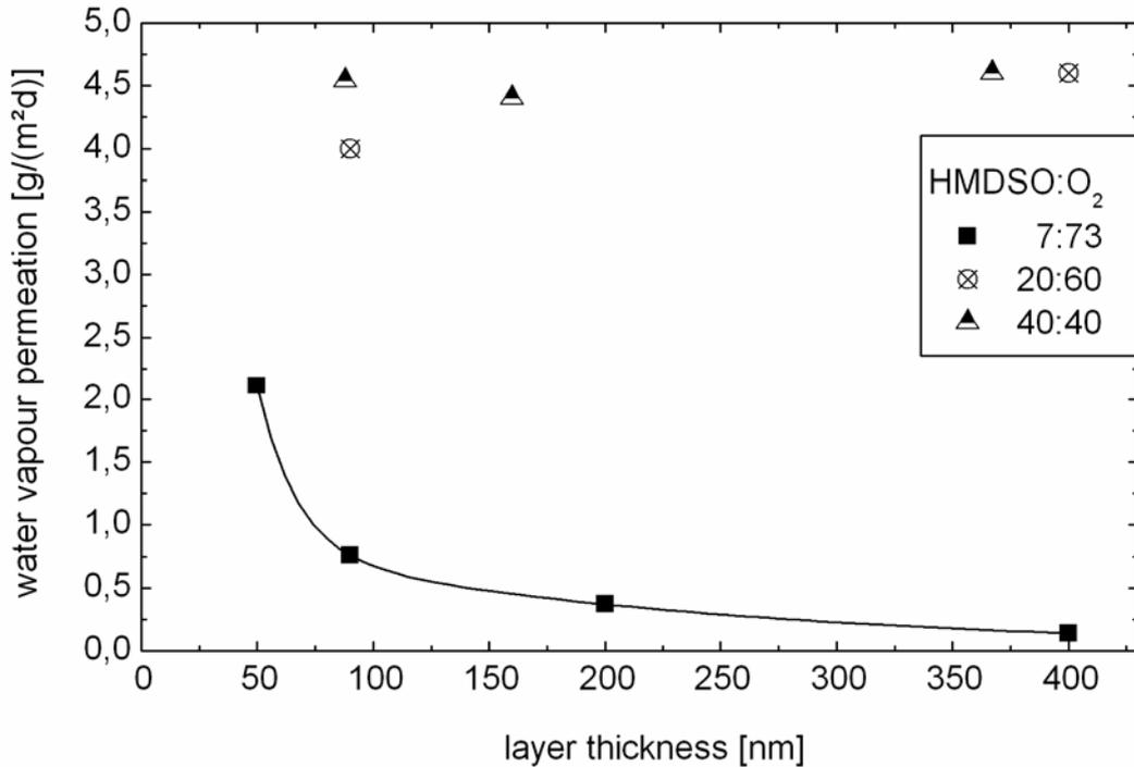
**Figure 7:** Water Vapor Transmission Rate of SiO<sub>x</sub>C<sub>y</sub> layers, deposited by magnetron PECVD (Substrate PET, 125 μm, WVTR measured at 38°C and 90% r.h.)
