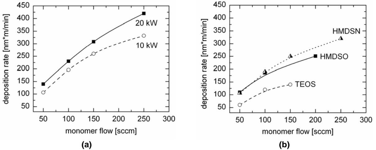
**Figure 4:** Deposition rate of the magnetron PECVD process in dependency on the monomer flow
