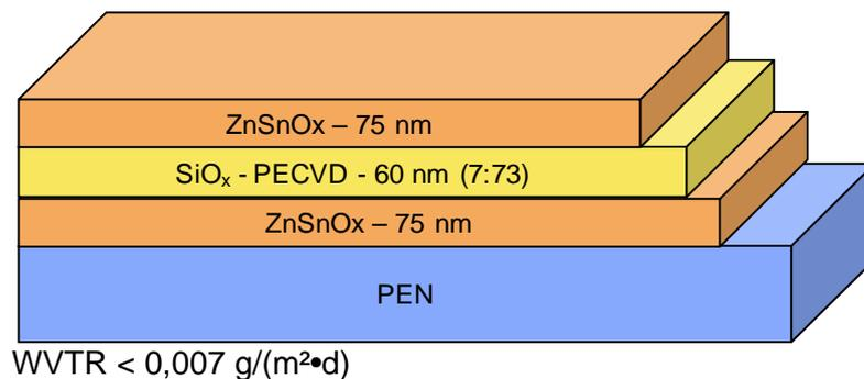
**Figure 9:** Three layer stack ZnSnOx (sputtering)/ SiO<sub>x</sub>C<sub>y</sub> (magnetron PECVD)/ ZnSnOx (sputtering) (substrate 75 μm PEN, WVTR measured at 38°C and 90% r.h.)
