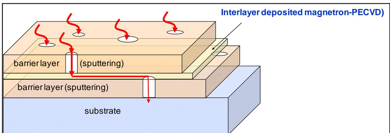
**Figure 1:** Basic multilayer barrier concept. The barrier layers are being deposited by dual magnetron sputtering whereas the interlayer is being deposited by magnetron PECVD.
