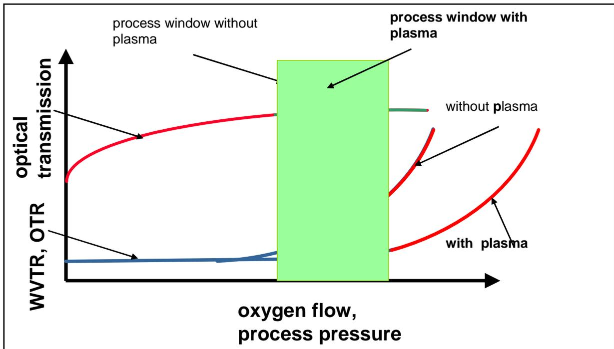
Figure 6: Process window of the reactive evaporation with and without plasma.
