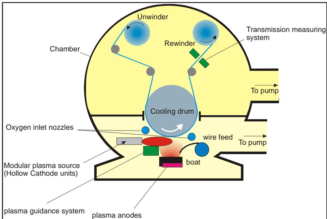
**Figure 1:** Basic configuration of a web coater for plasma-assisted reactive deposition of aluminum oxide on polymer films.
