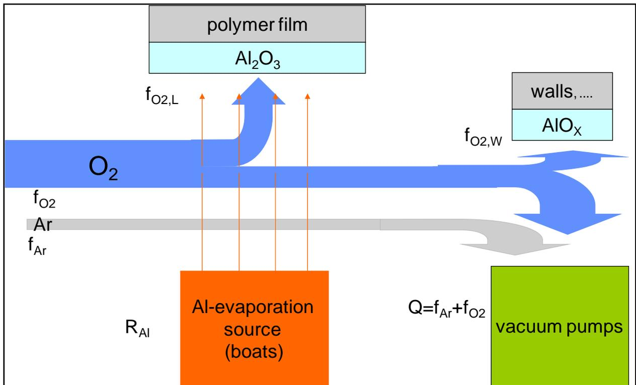
**Figure 2: Gas flow during reactive evaporation of aluminum**
