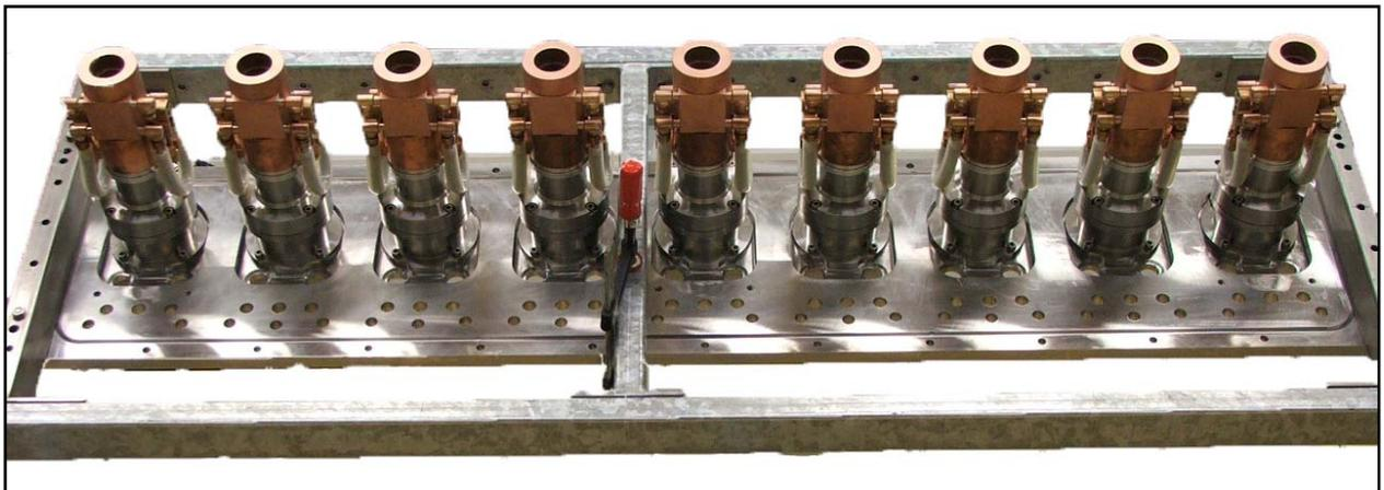
Figure 5: Plasma units mounted onto a bearing flange
