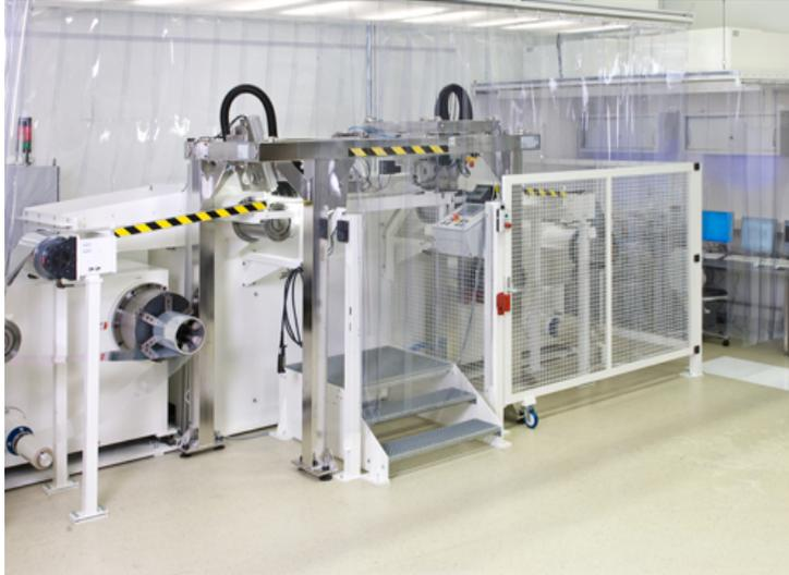
**Figure 4: Roll-to-Roll inspection system encased in a clean room carbine ISO6.**
