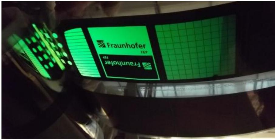
**Figure 10:** The photograph shows 100 x 100 mm<sup>2</sup> working OLED devices on a several meter long and 300 mm wide OLED demonstrator on 50  $\mu\text{m}$  ultra-thin glass.
