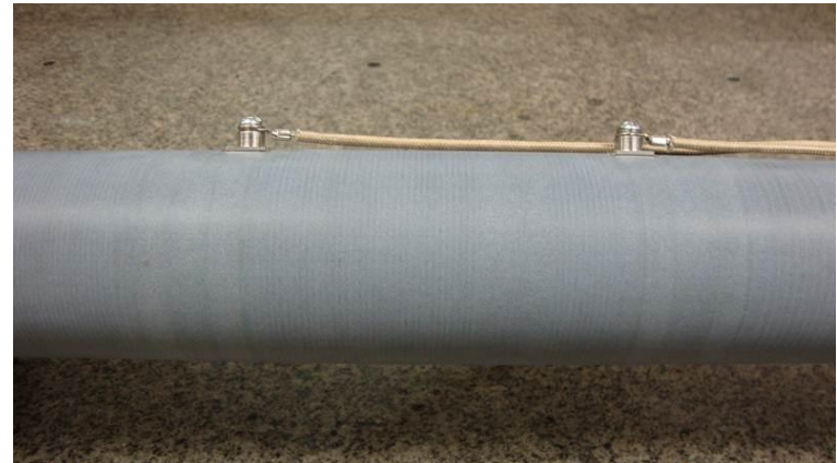
Low-profile connections with ring terminals and high-temperature (538°C/1000°F) hook-up wire
