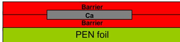
**Figure 3: Stack configuration for the bending test.**
