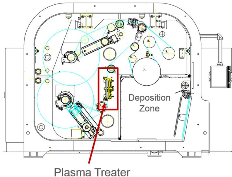
Figure 3: Cross section of the Bobst K5000 Metalliser. Indicated with the red box is the location of the plasma pretreater.
