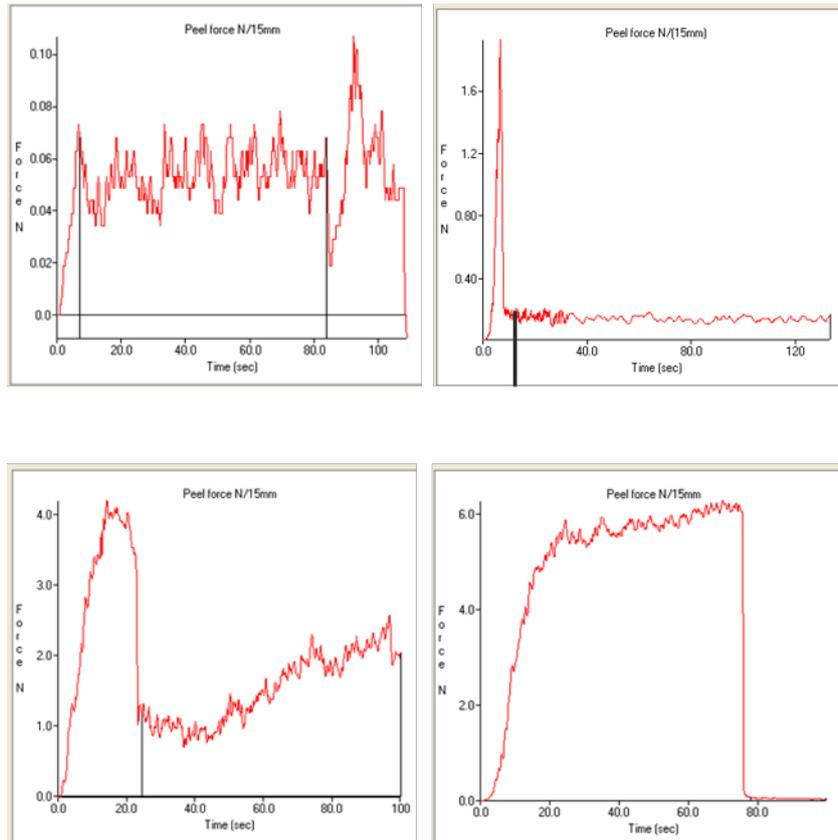
Figure 2: The four main peel force characteristics observed when performing peel tests.
