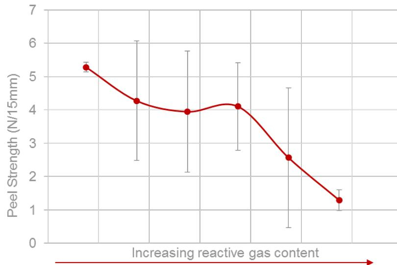
Figure 7: Relationship between peel strength and plasma oxygen content, decreasing in value as the oxygen content is increased.
