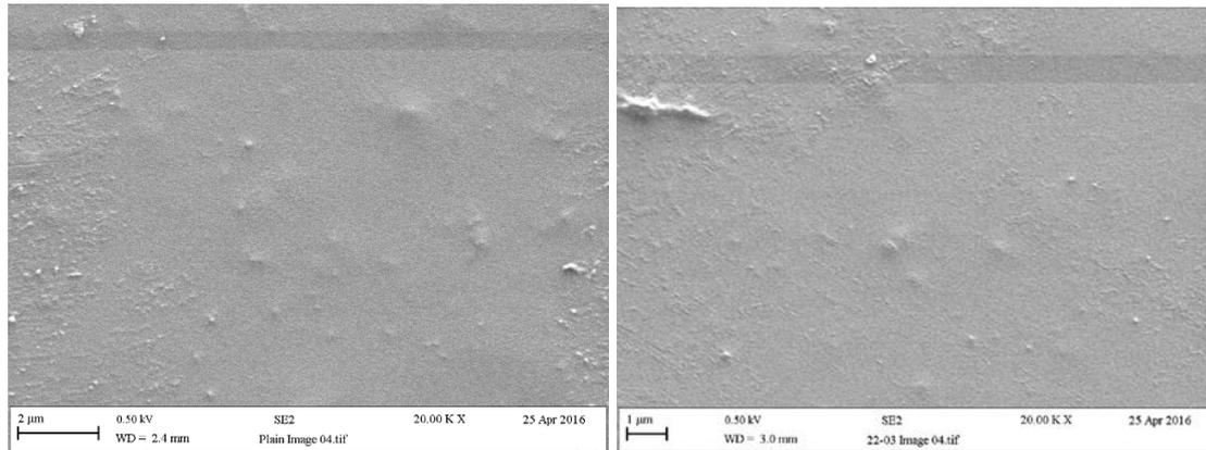
Figure 4: SEM micrographs (at 20,000 X magnification) displaying lack of difference between plain film (left) and plasma pretreated film at a production speed (right).
