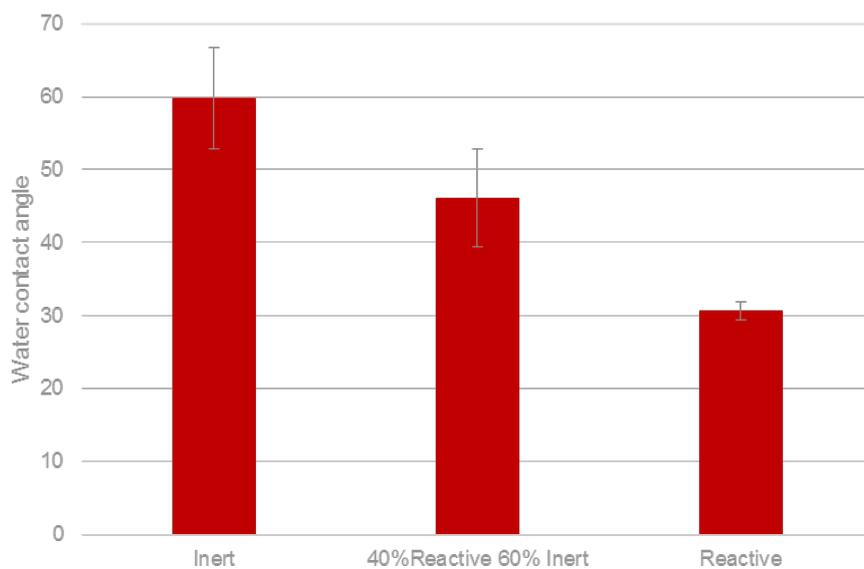
Figure 6: Water contact angles in relation to the Inert/Reactive gas ratio used for plasma treatment. The lower contact angle corresponds to a more wettable surface.
