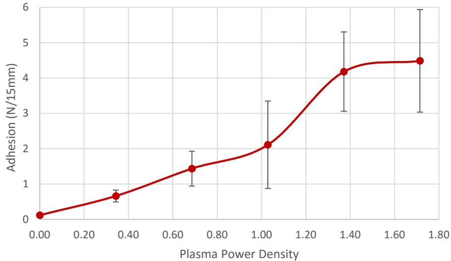
Figure 5: Plasma power density in relation to adhesion. High power density produced high adhesion samples.
