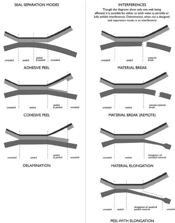
Figure 1: Peel test failures as explained by ASTM F88
