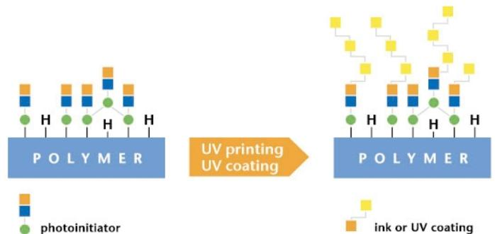
Figure 2. Post-Photografting Converting Process
