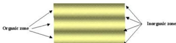
**Figure 3 Schematic of graded inorganic-organic ultra-high barrier coating.**
