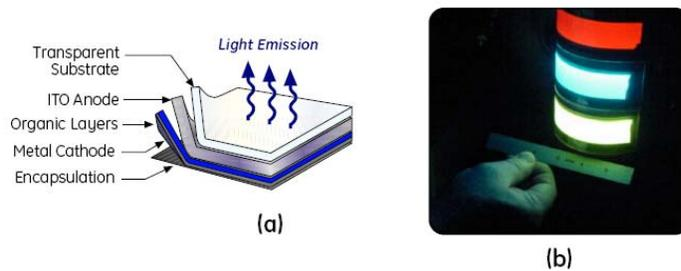
**Figure 1 (a) Schematic of an OLED device. (b) Flexible red, blue, and green OLEDs.**
