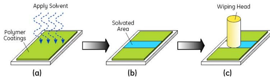
**Figure 5 Low cost R2R compatible solvent-assist-wipe patterning technique for organic thin film. (a) Apply solvent to the to-be-patterned area. (b) Solvent dissolves the organic coating material in applied area. (c) Use a polymeric wiping-head to physically remove organic material.**
